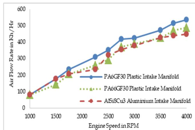
Figure 6. Variation of Air Flow Rate against Engine Speed
