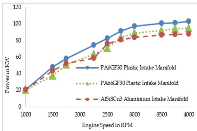
Figure 2. Variation of Power against Engine Speed
