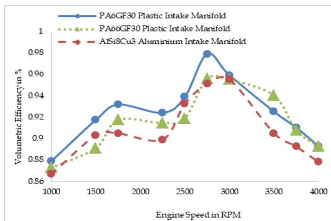
Figure 5. Variation of Volumetric Efficiency against Engine Speed
