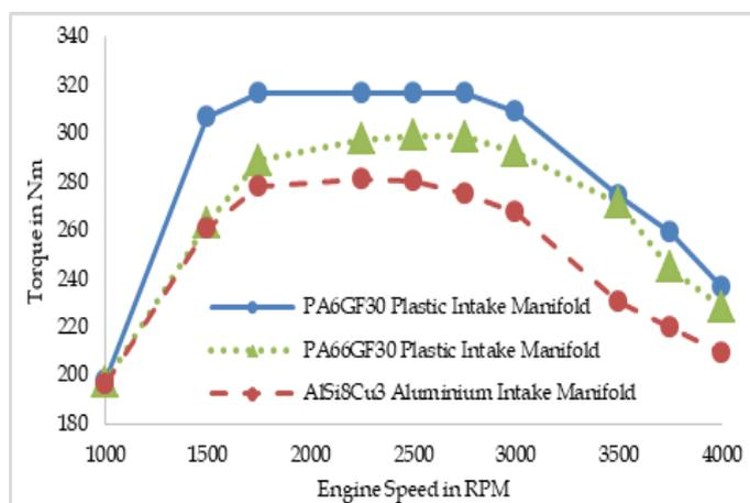
Figure 3. Variation of Torque against Engine Speed
