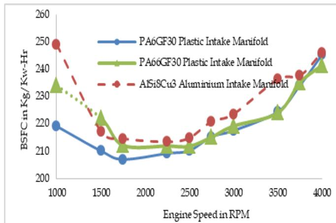
Figure 4. Variation of BSFC against Engine Speed
