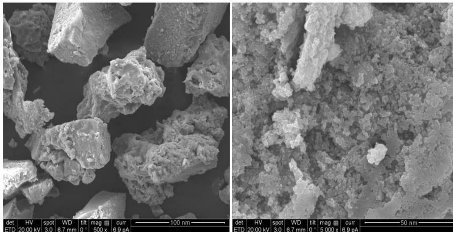
**Figure.4 SEM images of Silver nanoparticles at different magnification levels**
