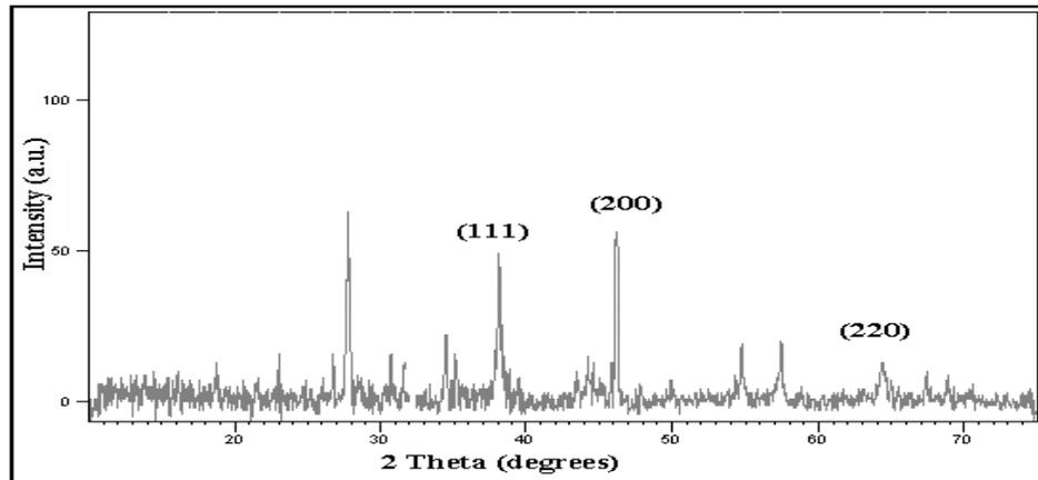
**Figure.3 XRD pattern of Silver nanoparticles**
