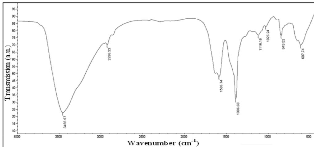
**Figure.2 FTIR spectrum of silver nanoparticles**
