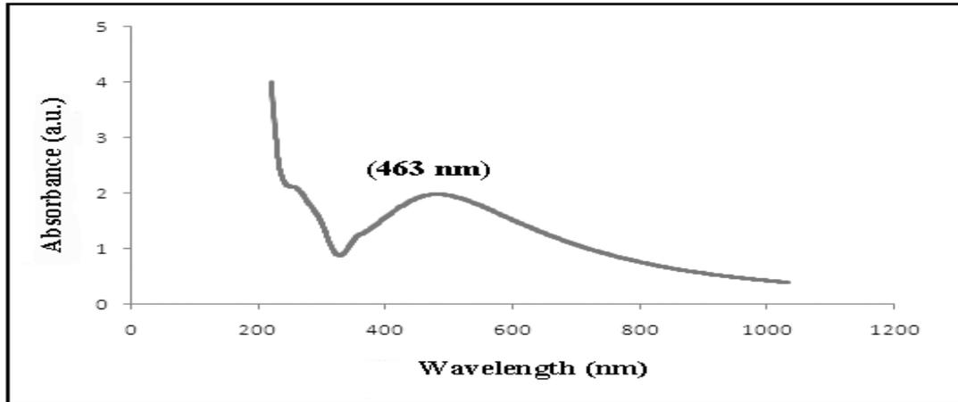
**Figure.1 UV-Vis spectrum of Silver nanoparticles**
