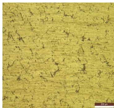
**Figure 15. Microstructure of the wire EDM surface of composite AA6063/SiC-G**
