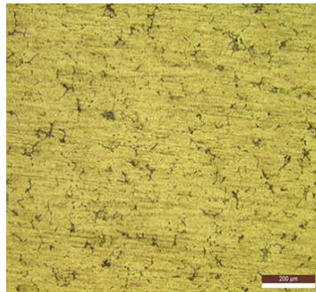
**Figure 14. Microstructure of the wire EDM surface of composite AA6063/SiC-B**
