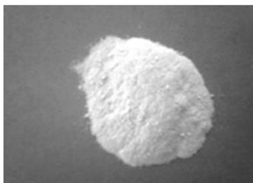
Figure 1.Mullite Powder before Ball Milling
