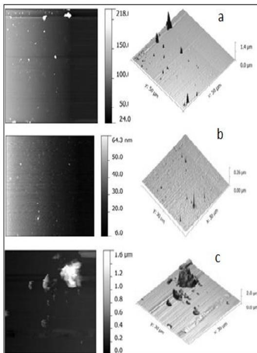
**Figure7. AFM 2D & 3D Image of Sample a, b & c at Different Ball Milling Intervals (75,100,150 hrs) from Top to Bottom**
