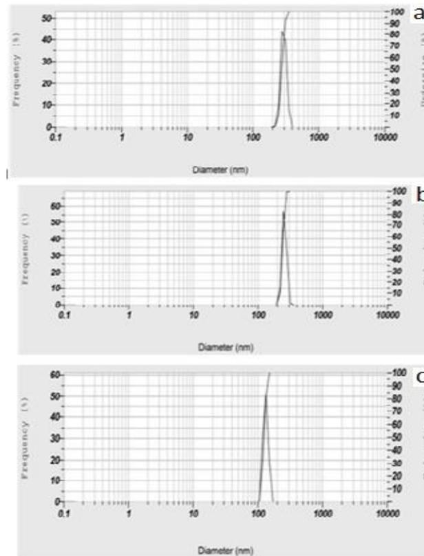
Figure 5. Particle Size Analyzer Sample a, b & c at Different Ball Milling Intervals (75,100,150 hrs) from Top to Bottom
