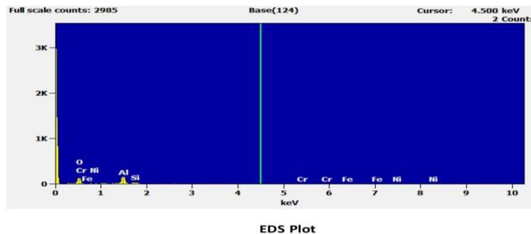
Figure 6.EDAX Spectrum of Mullite Nano Powder
