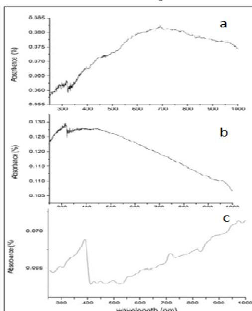
Figure 3. UV Spectrometer Plot for Sample a, b & c at Different Ball Milling Intervals (75,100,150 hrs) from Top to Bottom
