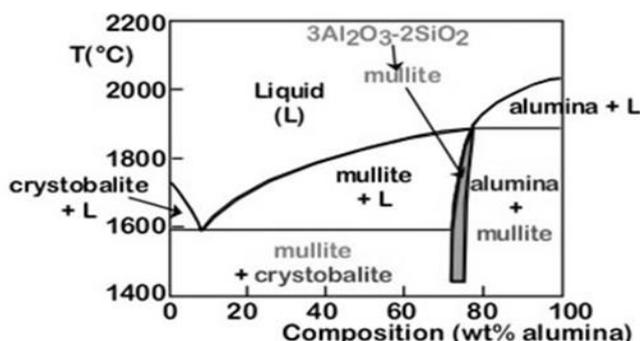
Figure 2.Multiphase Diagram of Mullite Powder
