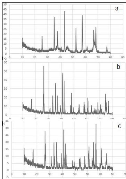
**Figure 4. XRD Spectrum for Sample a, b & c at Different Ball Milling Intervals (75,100,150 hrs) from Top to Bottom**
