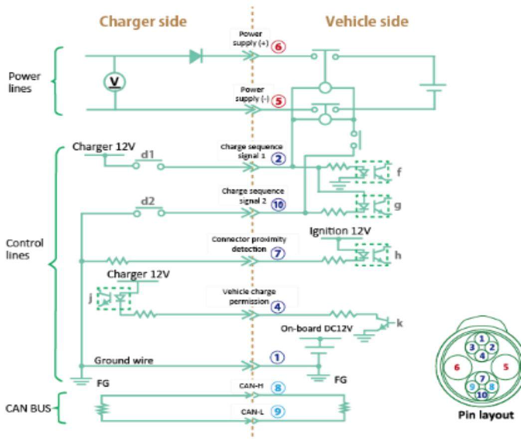
**Figure 6: Connector Interface Circuit**
