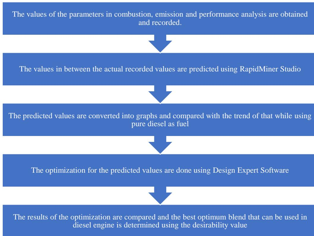
**Figure 3. Working procedure of the experiment**
