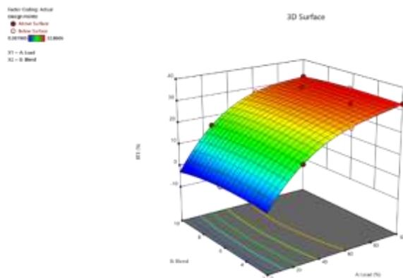
**Figure 4. Optimization Characteristics of Brake Thermal Efficiency**
