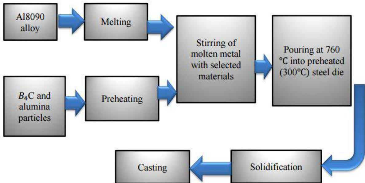
**Figure 2: Synthesis of composite**
