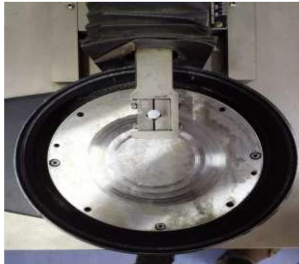
**Figure 3: Pin on Disc Setup Machine**
