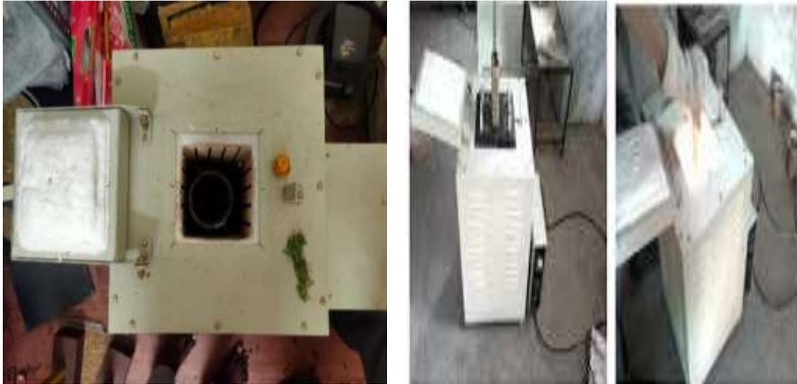
**Figure 1: Stir Casting Machine and Pre heating Setup**
