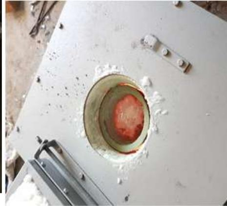
Figure 1B :Al 6061 melted at 800°C
