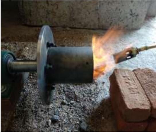
Figure 1C :preheating of centrifugal mould at 400°C
