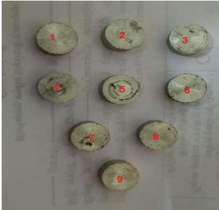
Figure 3: FGM thermal conductivity specimen
