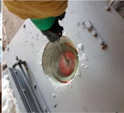
Figure 1D: Al melts mixing with reinforcements
