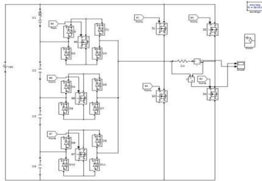
**Figure 7: Simulation diagram of the nine-level inverter with a switched capacitor.**
