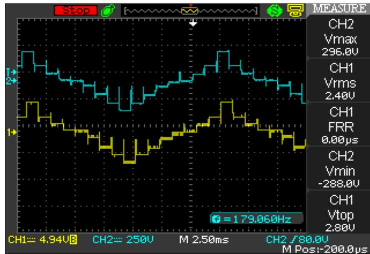
Figure 14: Nine level output voltage & current
