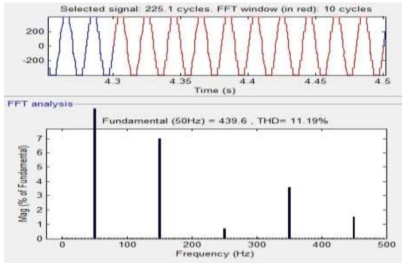
Figure 9: Total harmonic distortion of the nine-level output voltage.
