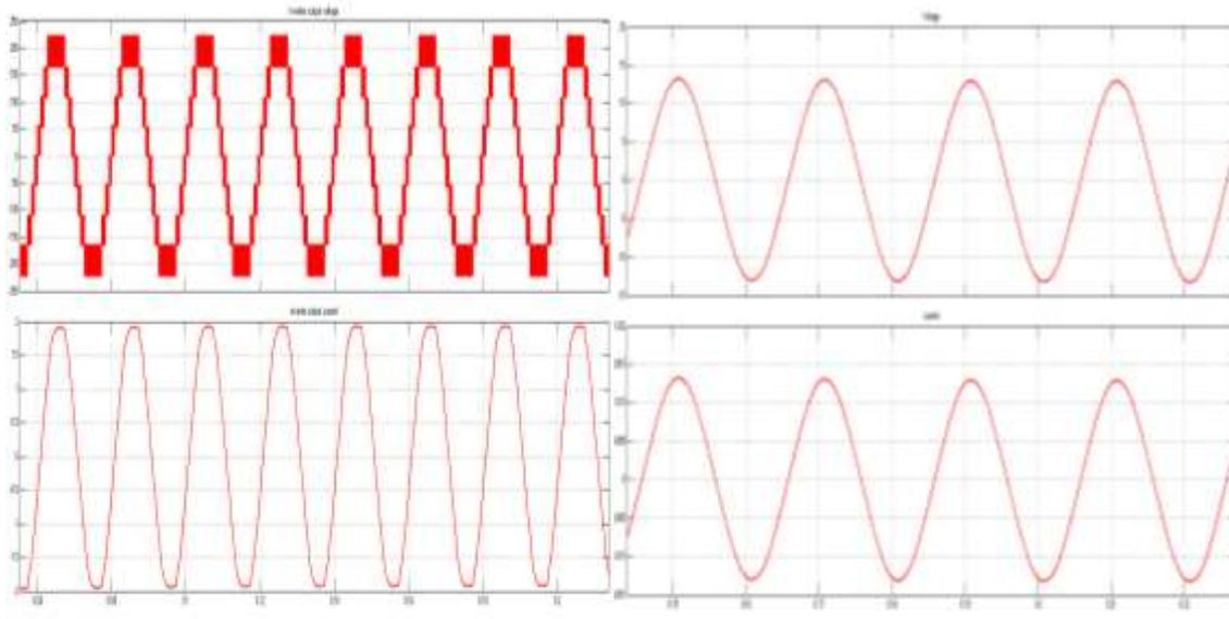
**Figure 12: a) Nine-level inverter output voltage and current waveform before filtering. b) Nine-level inverter output voltage and current waveform after filtering.**
