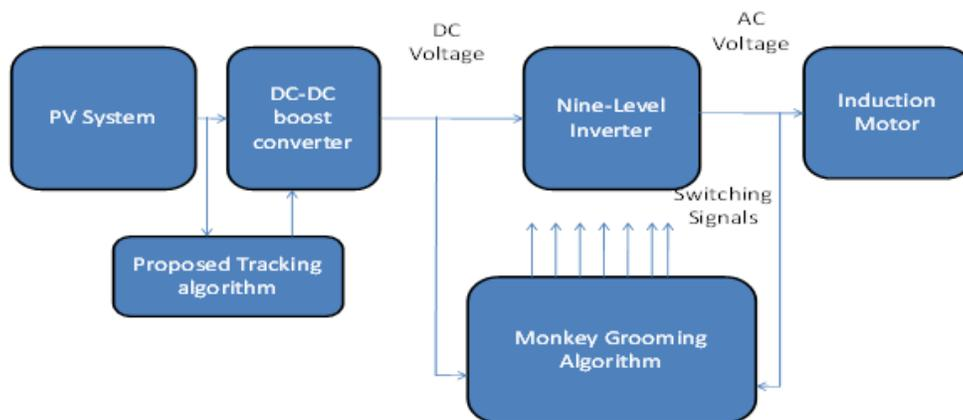
**Figure 1: Block diagram of the overall system**
