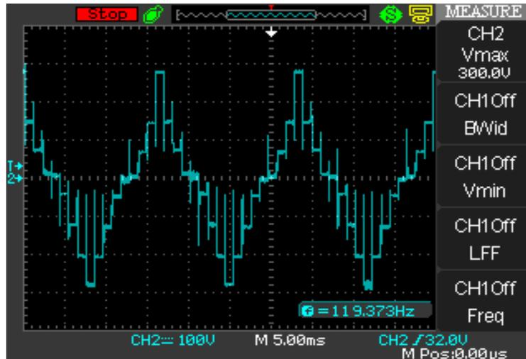
Figure 13: Nine level output voltage
