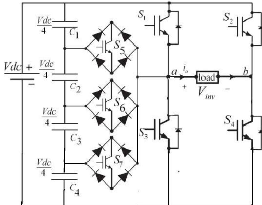
**Figure 2: Topology of Single-phase nine-level inverter circuit**
