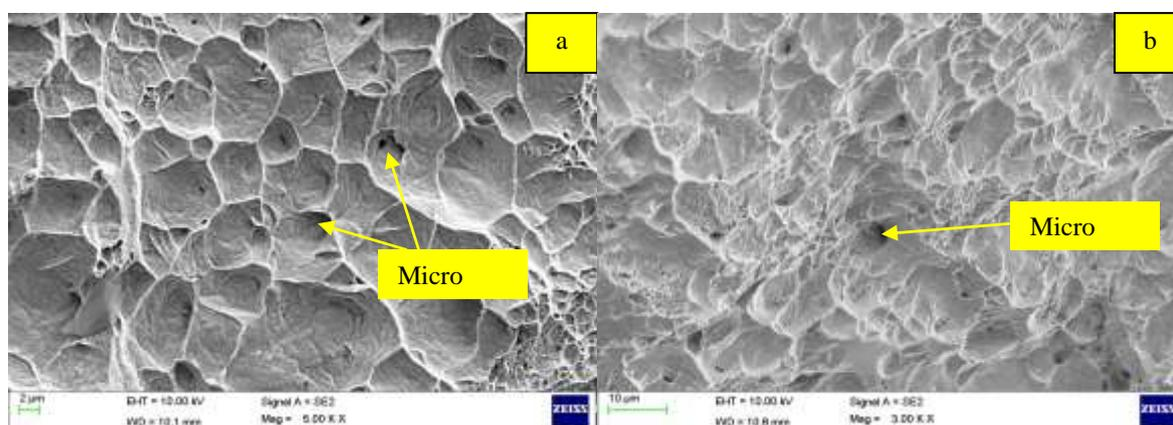
**Figure 12. SEM Fractograph of impact failure of PCGTAW (a) ERNiCrFe-7; (b) ERNiCr-3**
