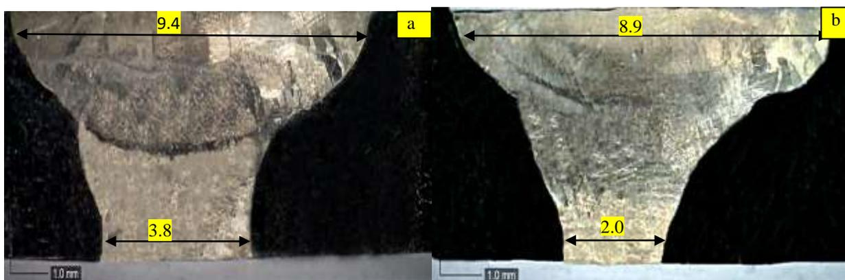
Figure 3. Macrostructure image of the weld joints (a) PCGTAW ERNiCrFe-7; (b) PCGTAW ERNiCr-3
