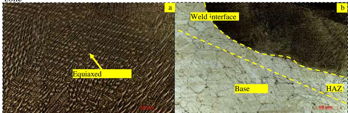
**Figure 5. Optical microscopy of PCGTAW joints using ERNiCr-3 (a) Weld center; (b) Weld Interface.**
