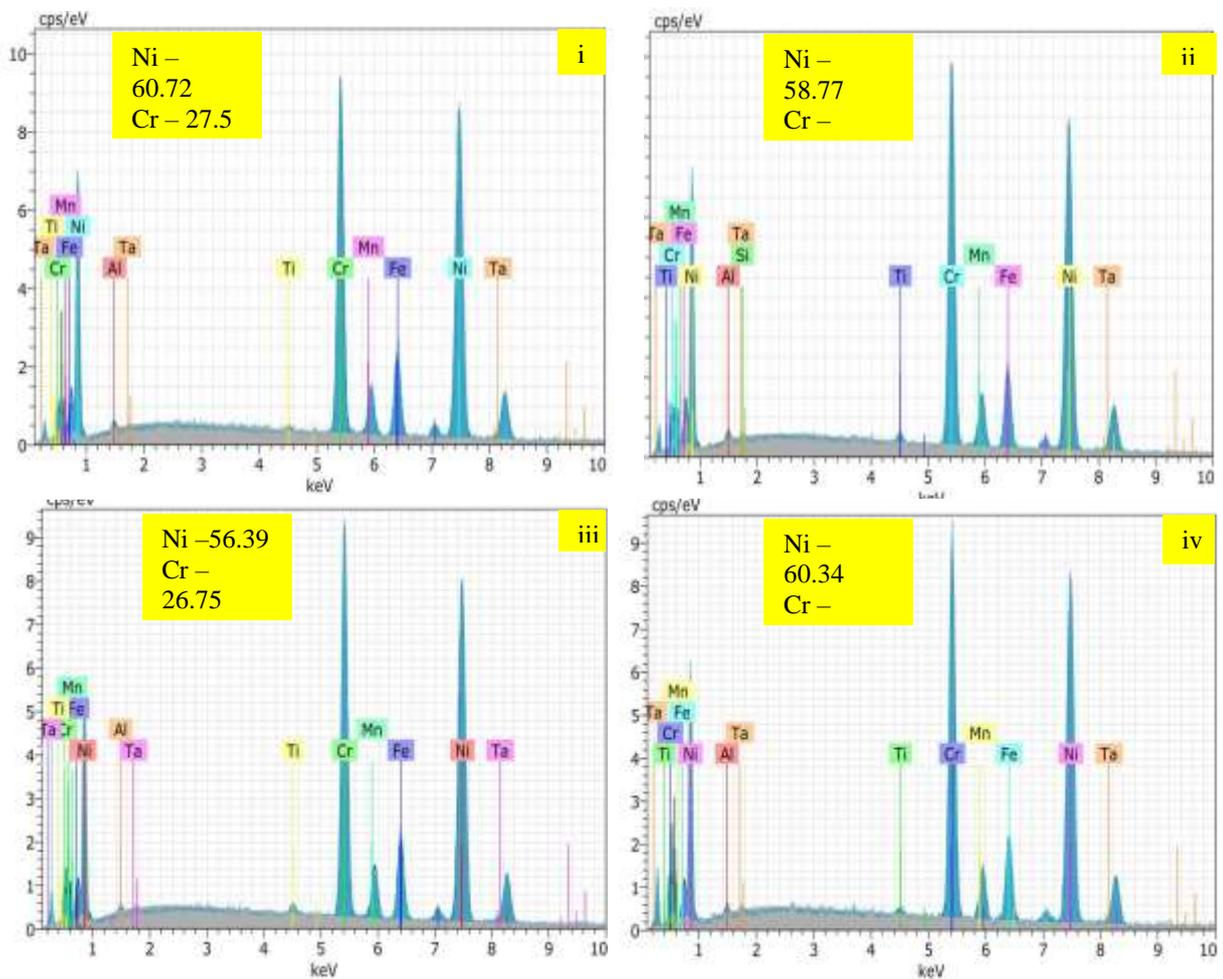
Figure 6. SEM/EDS analysis for ERNiCrFe-7 PCGTAW (a) SEM weld center ; (b) SEM weld interface ; (i) EDS of weld center dendritic core ; (ii) EDS of weld center interdendritic region ; (iii) EDS of weld interface dendritic core and (iv) EDS of weld interface interdendritic region
