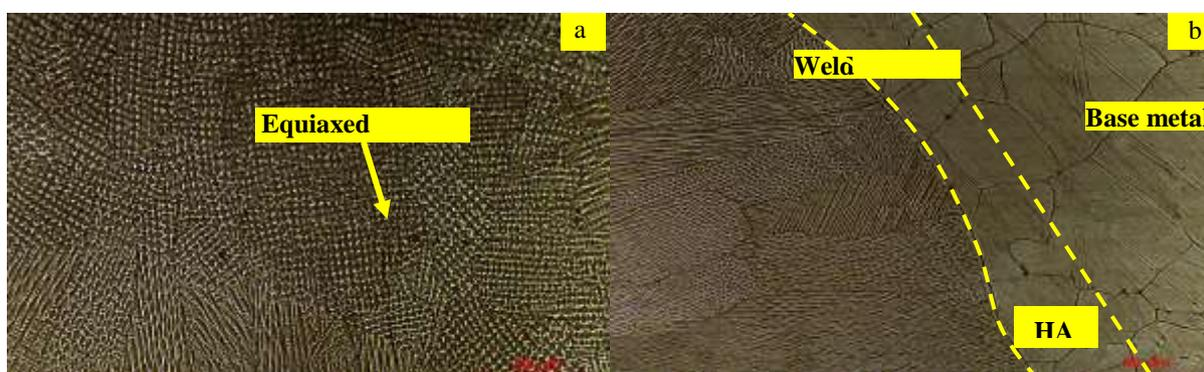
Figure 4. Optical microscopy of PCGTAW joints using ERNiCrFe-7 (a) weld center; (b) Weld Interface.
