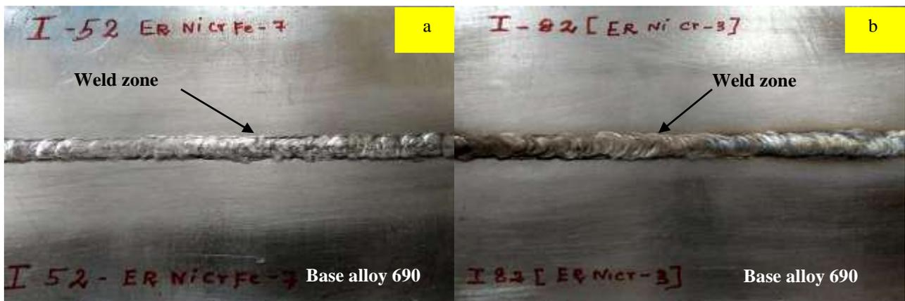
Figure 1. Photographic images of weldments made with (a) PCGTAW ERNiCrFe-7; (b) PCGTAW ERNiCr-3
