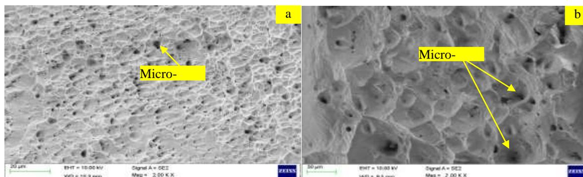
**Figure 10. SEM Fractograph of tensile failure of PCGTAW (a) ERNiCrFe-7; (b) ERNiCr-3**
