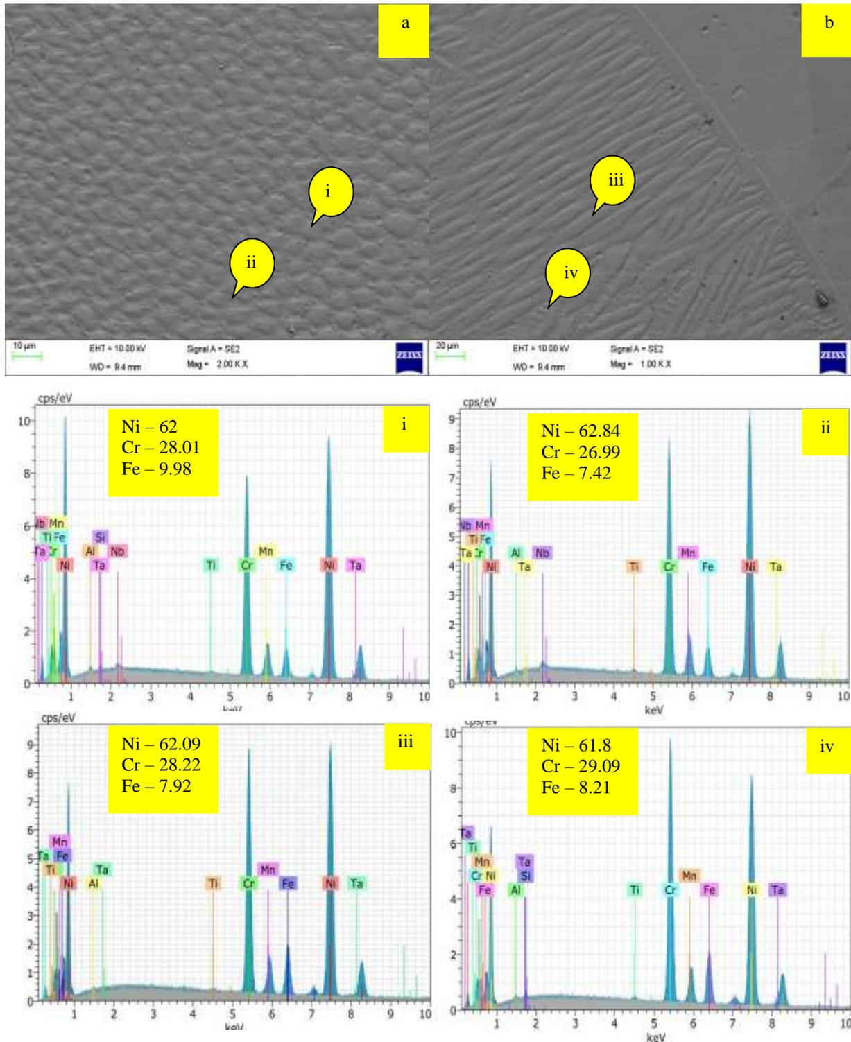
**Figure 7. SEM/EDS analysis for ERNiCr-3 PCGTAW (a) SEM weld center ; (b) SEM weld interface ; (i) EDS of weld center dendritic core ; (ii) EDS of weld center interdendritic region ; (iii) EDS of weld interface dendritic core and (iv) EDS of weld interface interdendritic region**
