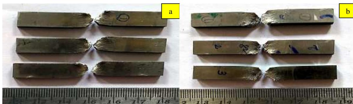
**Figure 11. Photographs of impact test of fractured specimen (a) PCGTAW ERNiCrFe-7; (b) PCGTAW ERNiCr-3**
