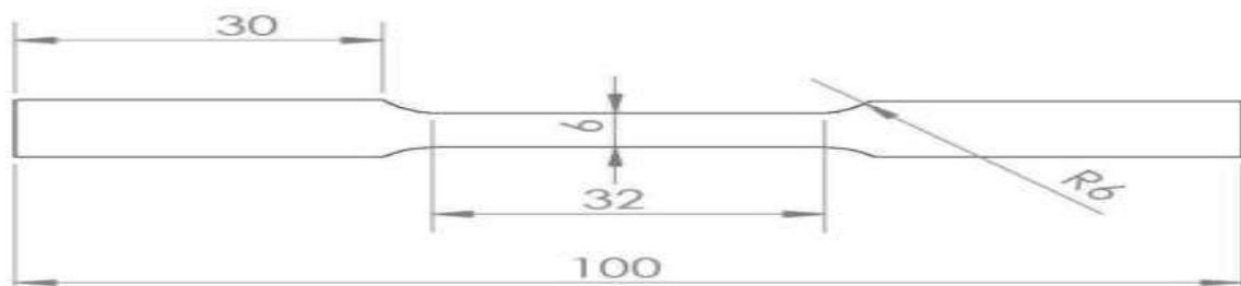
Figure 2. Schematic diagram showing the dimensions of tensile specimen
