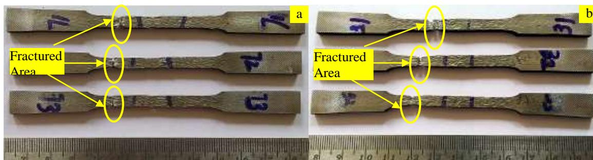
**Figure 9. Photographs of tensile test of fractured specimen (a) PCGTAW ERNiCrFe-7; (b) PCGTAW ERNiCr-3**
