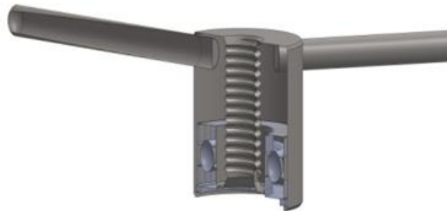
Figure 1. Cross section of handling wheel
