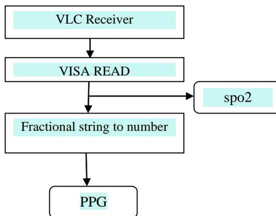
**Figure 4. Flowchart for PPG signal and spo2 reception**
