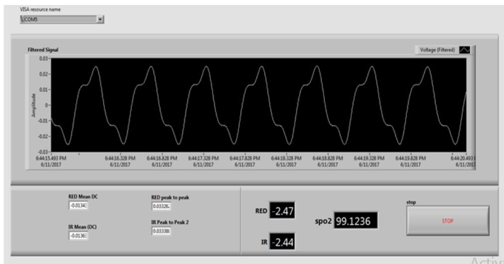
Figure 6. Transmitted PPG signal and spo2
