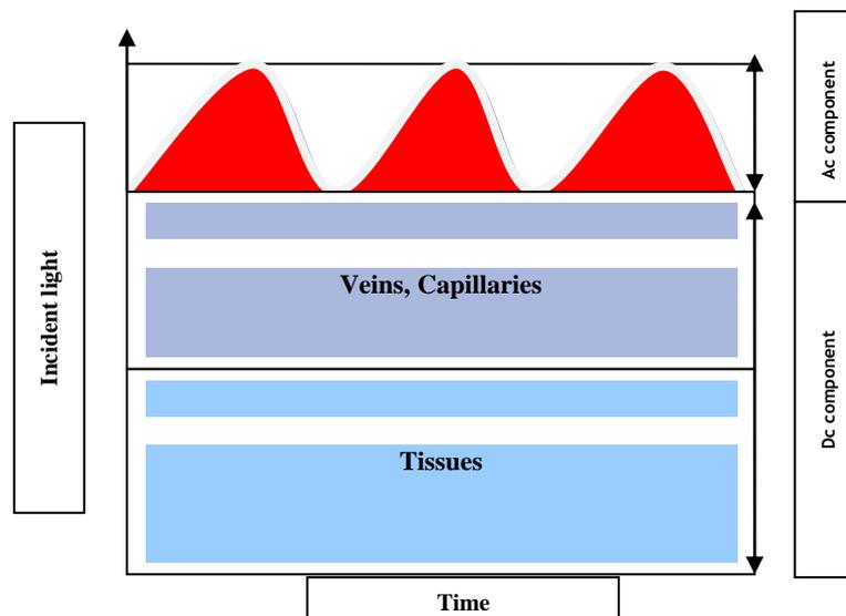
**Figure 1. Light absorption in finger**
