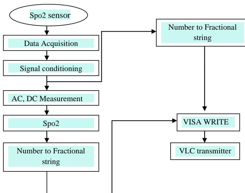
Figure 2.Flowchart for PPG signal and spo2 transmission
