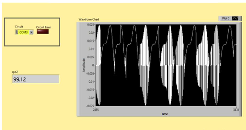
Figure 7. Received PPG signal and spo2
