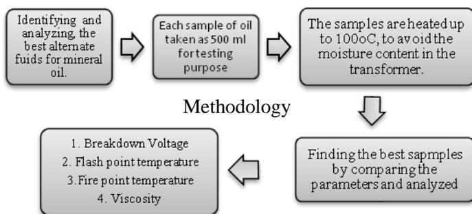
Figure 3. Methodology of liquid analysis
