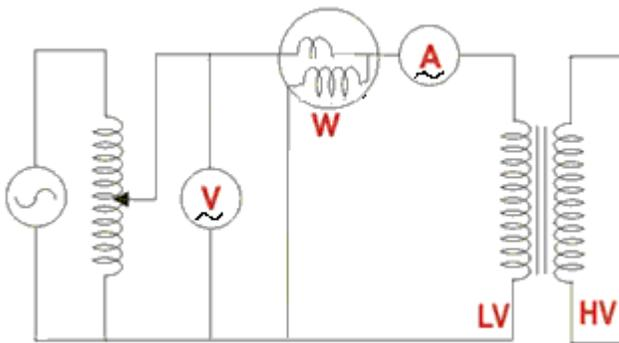
Figure 1. Circuit diagram for O.C test.
