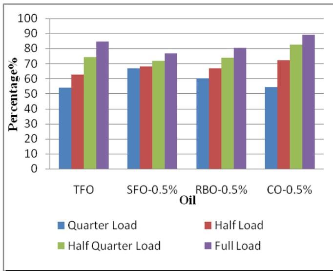
**Figure 7.** By Comparing the efficiency under various load condition in transformer with TFO and SFO, RBO & CO with and without antioxidant via bar chart
