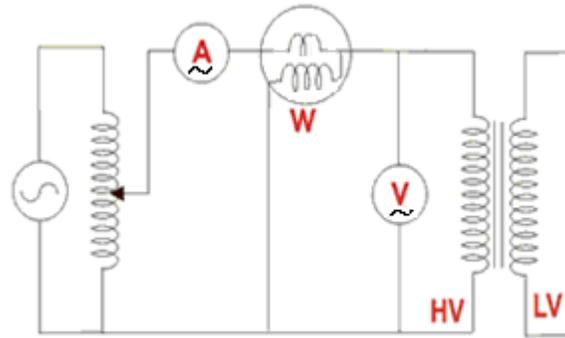
Figure 2. Circuit diagram for S.C test
