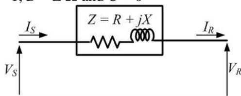
**Fig 2. Short transmission line representation.**
