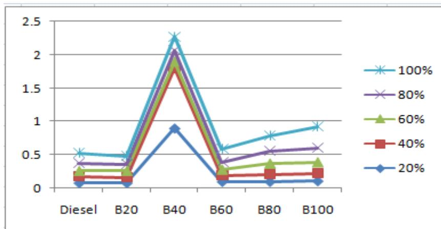
**Figure 12 Load vs CO Emission**
