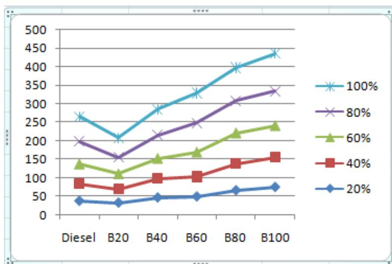
**Figure 14 Load vs HC Emission**
