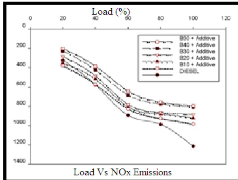
Figure 7 Load vs Nitrogen Oxide Emissions of pumpkin seed
