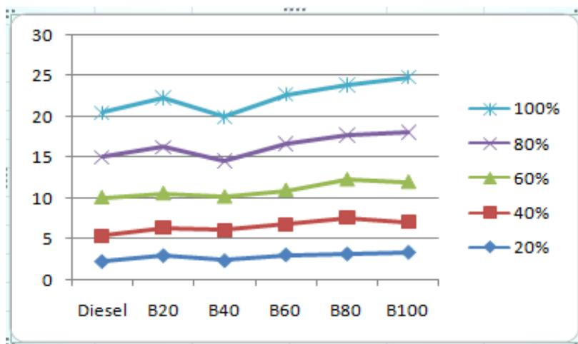
**Figure 13 Load vs CO<sub>2</sub> Emission**
