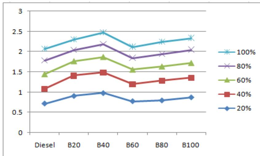
Figure 10 Load vs BSFC
