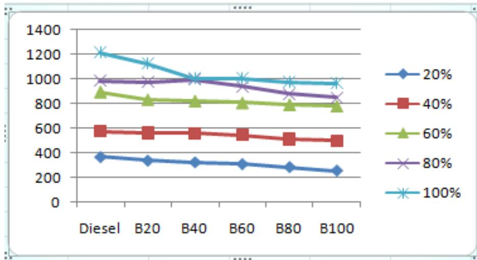
**Figure 11 Load vs NOx Emission**
