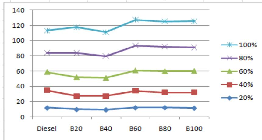
Figure 9 Load vs BTE
