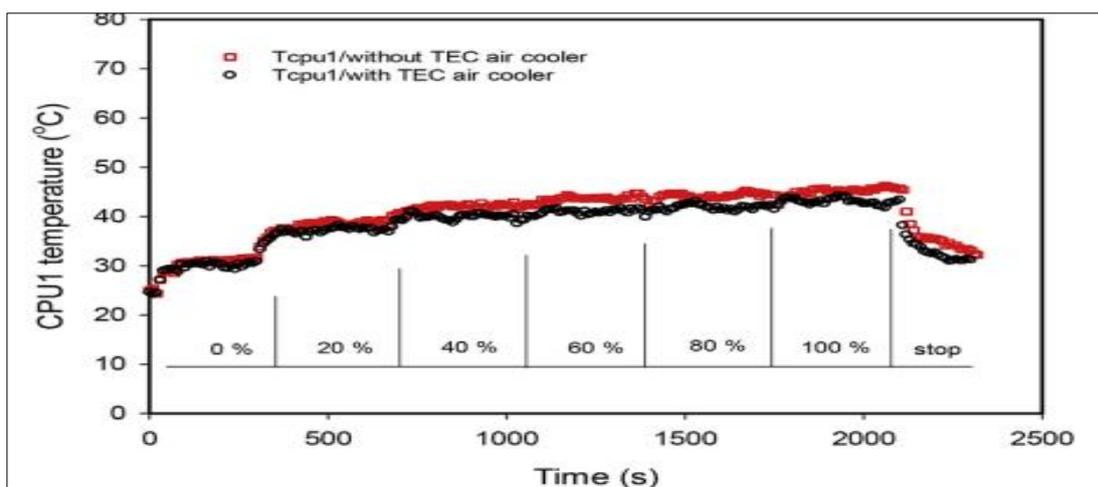
**Fig.2 Illustration of non-performance of conventional air cooling as in [2]**
