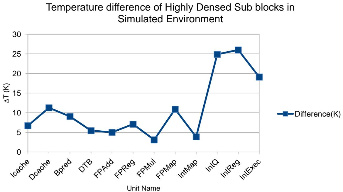
**Fig.4.b Demonstration of  $\Delta T$  of specific hotspots**
