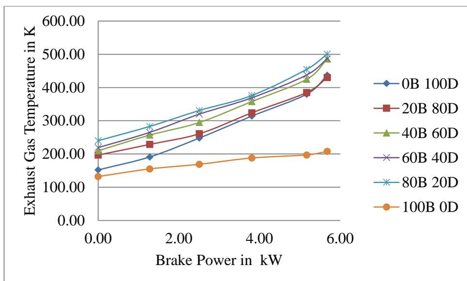
**Figure 3.4 Exhaust Temperature Vs BP**
