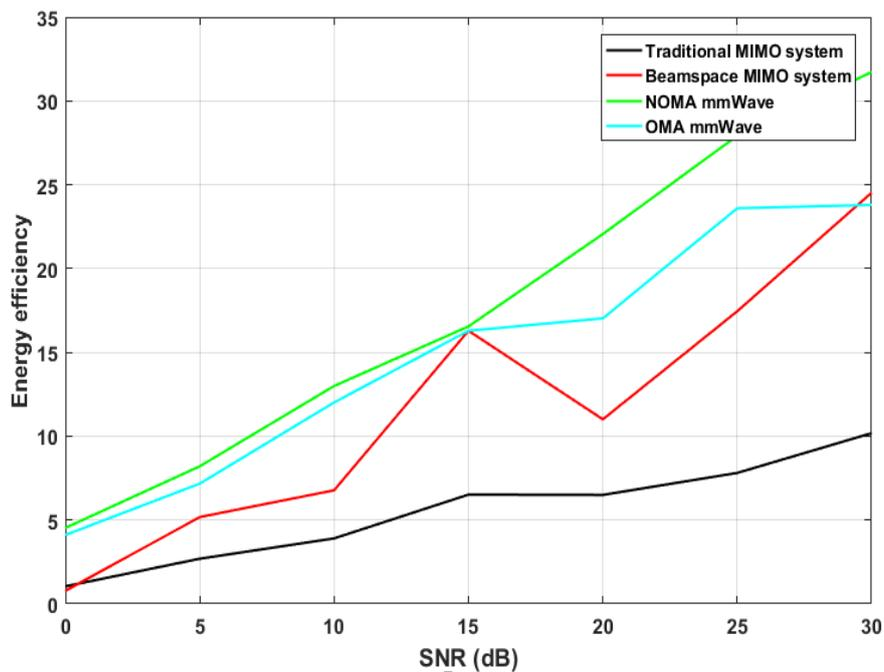
**Figure 3. Energy Efficiency Vs SNR**
