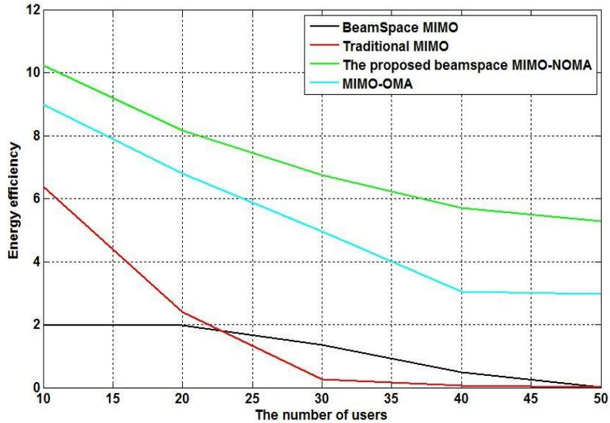
**Figure 4. Energy efficiency Vs Users K**
