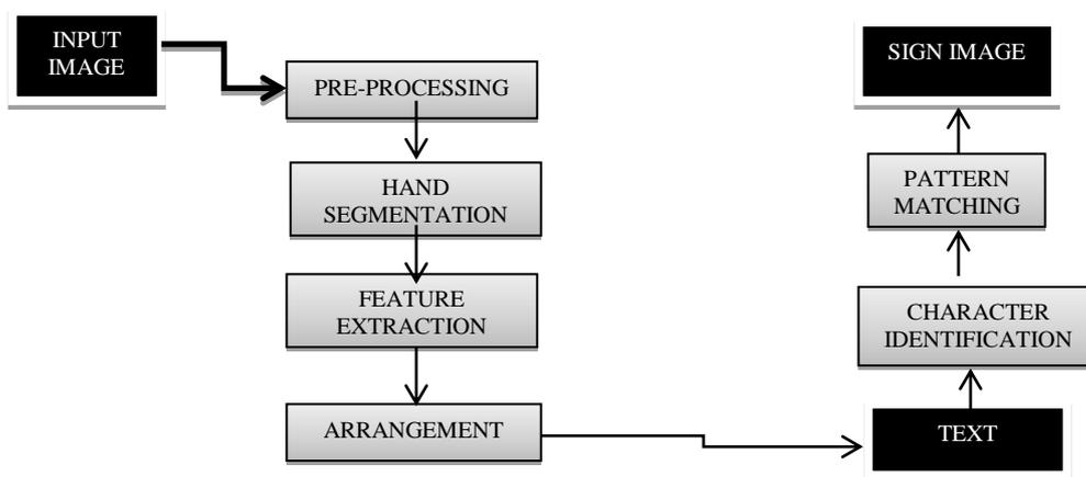
In this approach, the movement of the hand is captured by a camera. The image contains background pixels other than the hand, as a hand will never fill a perfect square. The system captures the hand signs image from the unique image and recognize the skin-colored area and acquires the hand divided out from the rest of the background. Next, the binary mask for skin pixels is constructed
