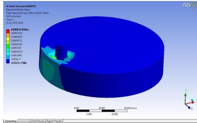
Figure 12. Wear Strain of PU/MoS<sub>2</sub>/TiO<sub>2</sub> (89/10/1)
