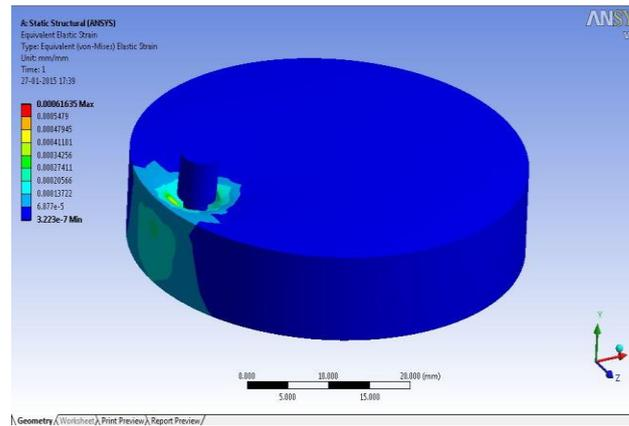
**Figure 10. Wear Strain of PU/MoS<sub>2</sub>/TiO<sub>2</sub> (92.5/7/0.5)**
