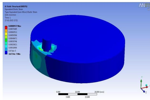
Figure 14. Wear Strain of PU/MoS<sub>2</sub>/TiO<sub>2</sub> (78.5/20/1.5)
