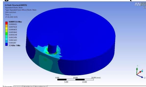
Figure 6. Wear Strain of PU / MoS<sub>2</sub> (90/10)
