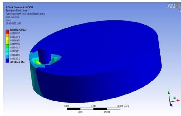
Figure 4. Wear Strain of PU / MoS<sub>2</sub> (93/7)
