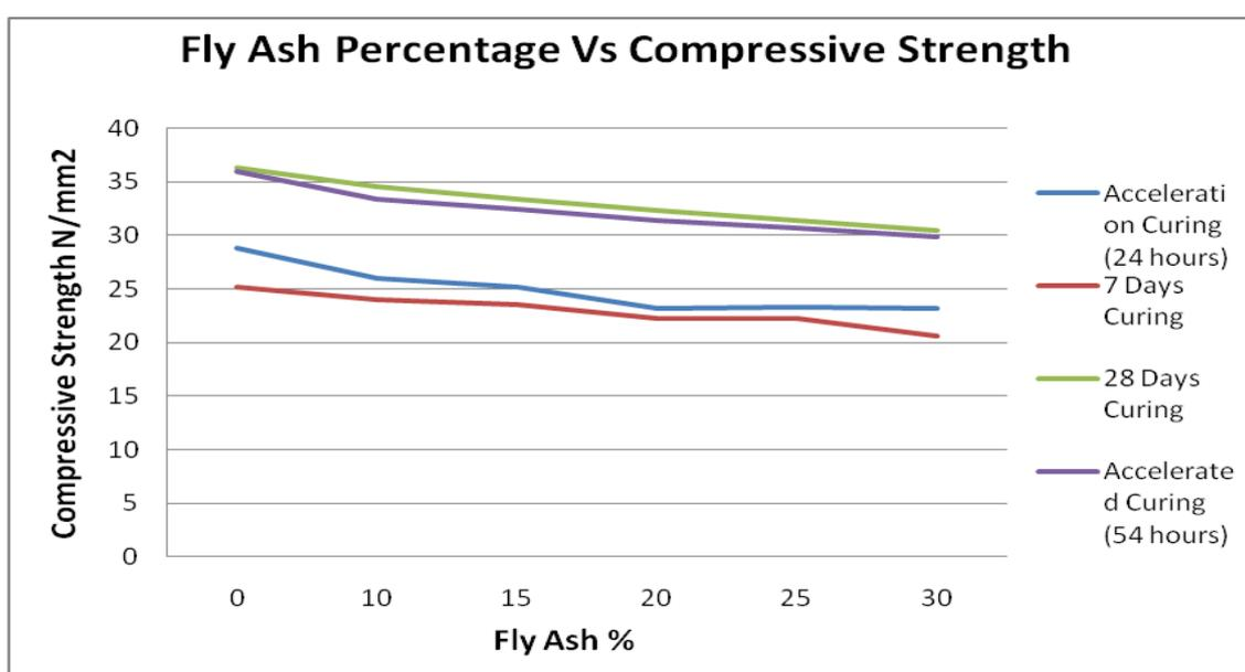
**Figure:** Showing the compressive strength in different curing with varying fly ash %
