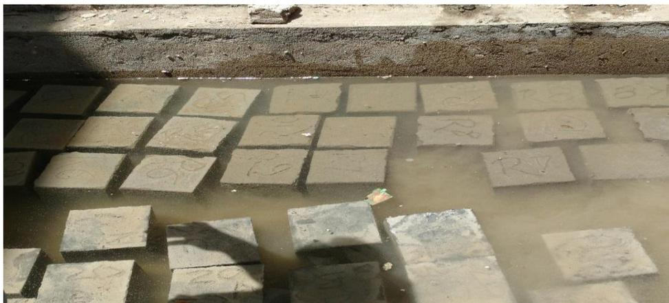
**Figure:** Curing of 66 cubes in Curing pond constructed outside of concrete lab in open air.
