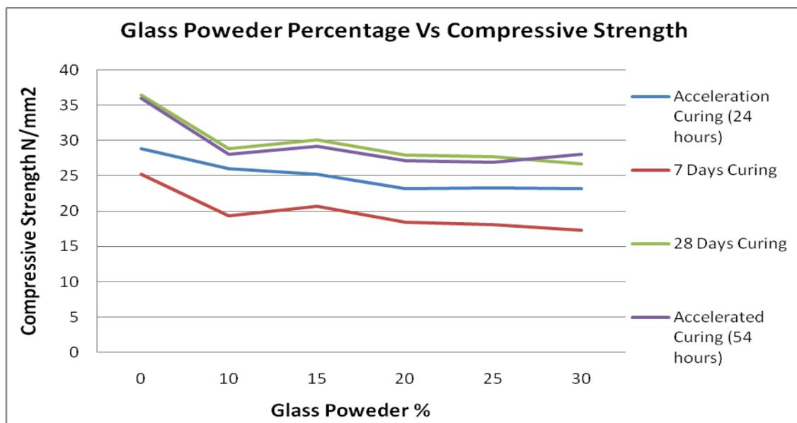
**Figure:** Showing the compressive strength in different curing with varying Glass Powder %
