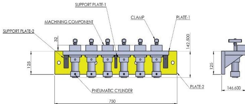
Fig 2.2.2 Fixture design with parts name
