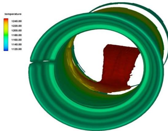
**Figure 5.** Simulated temperature distribution during filling of a pipe in a front view. The hot inflowing melt (in red colour) is distributed along the inner tube-shaped steel mould due its rotation.
