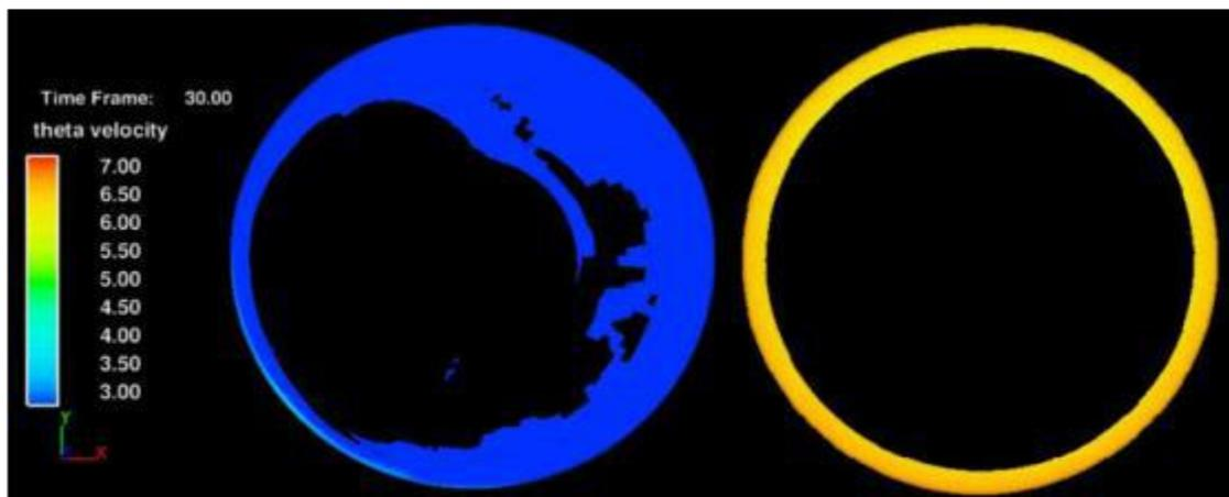
**Figure 4.** The simulation with low surface roughness (left) shows an unstable melt curtain, the simulation with an appropriate surface roughness (right) shows a stable melt following the looping condition.
