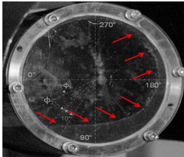
**Figure 3.** Shape of the free surface of the Rose's alloy at a selected revolution speed
