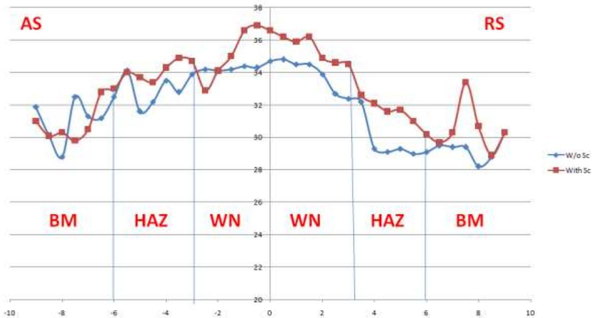
Fig. 5. Hardness survey of the welded samples.
