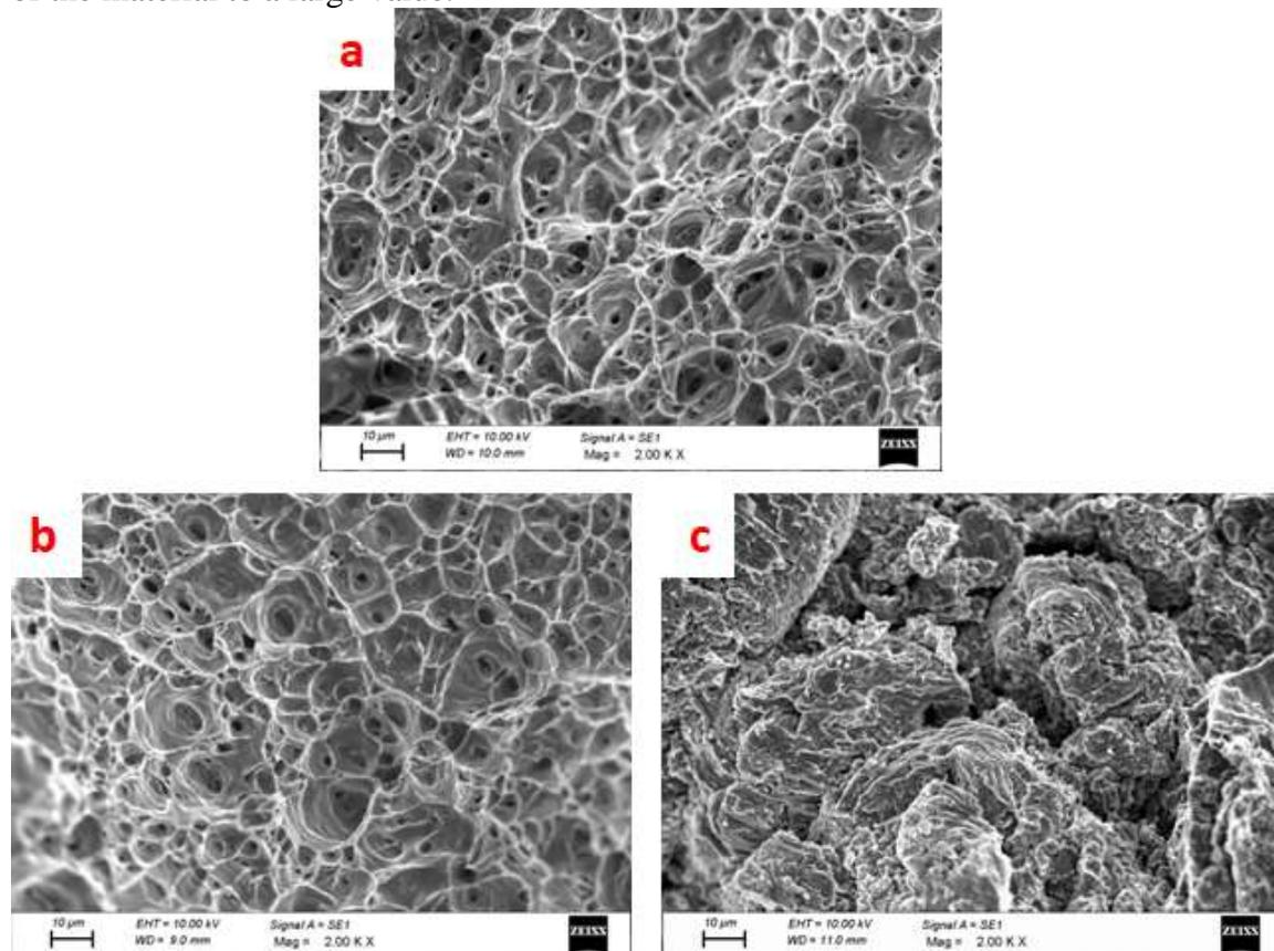
Fig. 4. Fractography images (a) Base metal AA1200 (b) without scandium insert (c) with scandium insert
