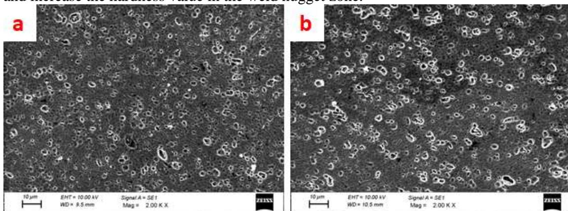
Fig. 2. SEM images of the weld nugget (a) Without scandium insert (b) with scandium insert
