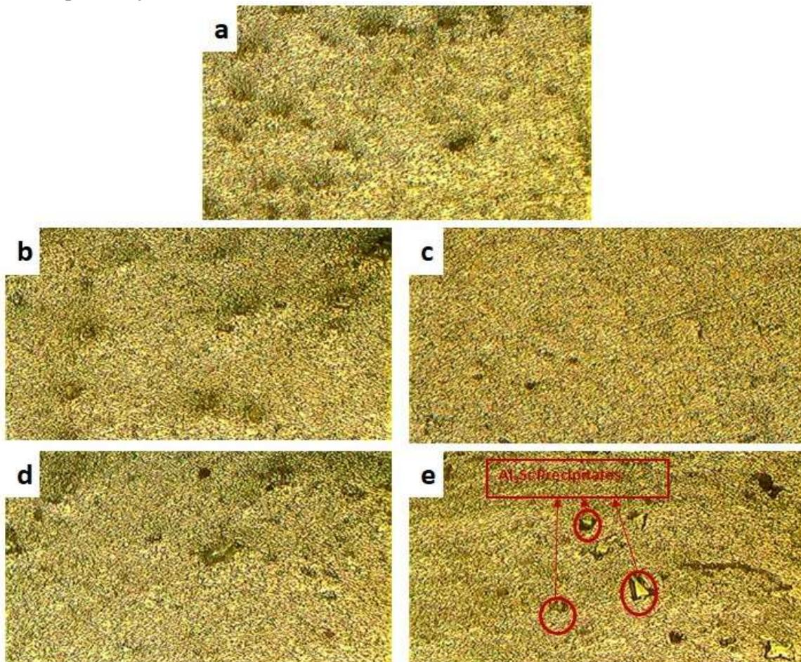
Fig. 1 Optical Microscopy (100 X Magnification) – (a) Base Metal, (b) HAZ of FSWed AA1200 without Sc insert, (c) HAZ of FSWed AA1200 with Sc insert, (d) Weld Nugget of FSWed AA1200 without Sc insert, (e) Weld Nugget of FSWed AA1200 with Sc insert.
