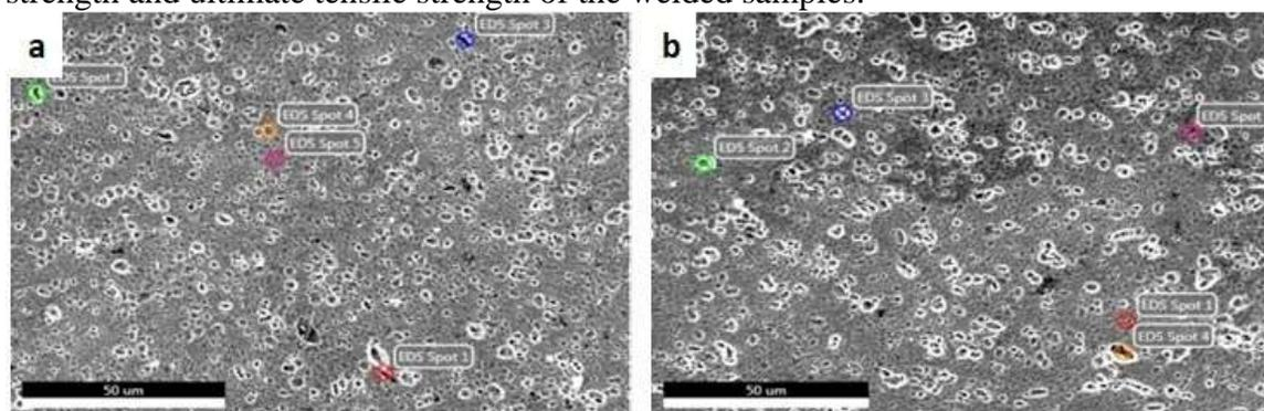
Fig. 3. SEM EDX images at the weld nugget (a) Without scandium insert (b) with scandium insert.
