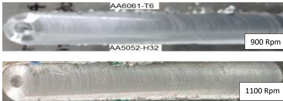
Figure. 1 Surface Aspects of Dissimilar Weld Prepared by FSW at Various Rotation rates
