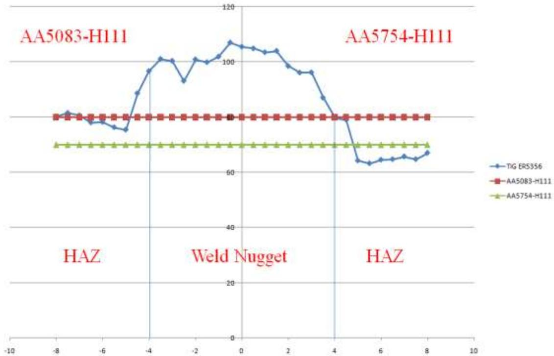
Fig. 4. Vickers Hardness Plot of the base metals and welded sample.
