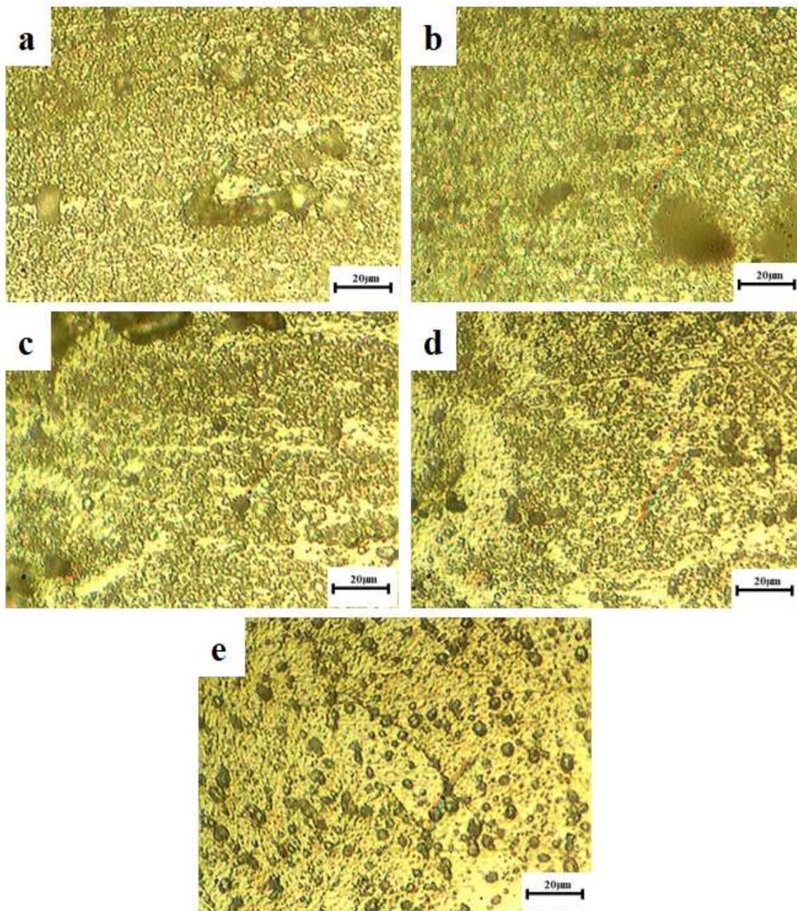
Fig. 1. Optical Microscopy (a) AA5083 Base Material (b) AA5754 Base Material (c) AA5083 HAZ (d) AA5754 HAZ (e) Weld Zone
