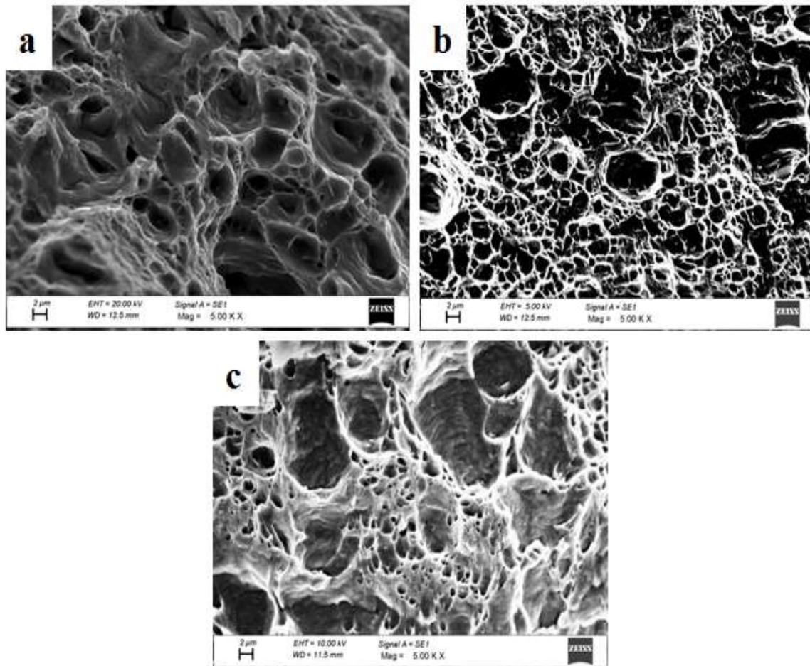
Fig. 3. Fractography (a) AA5083 Base Material (b) AA5754 Base Material (c) Welded sample
