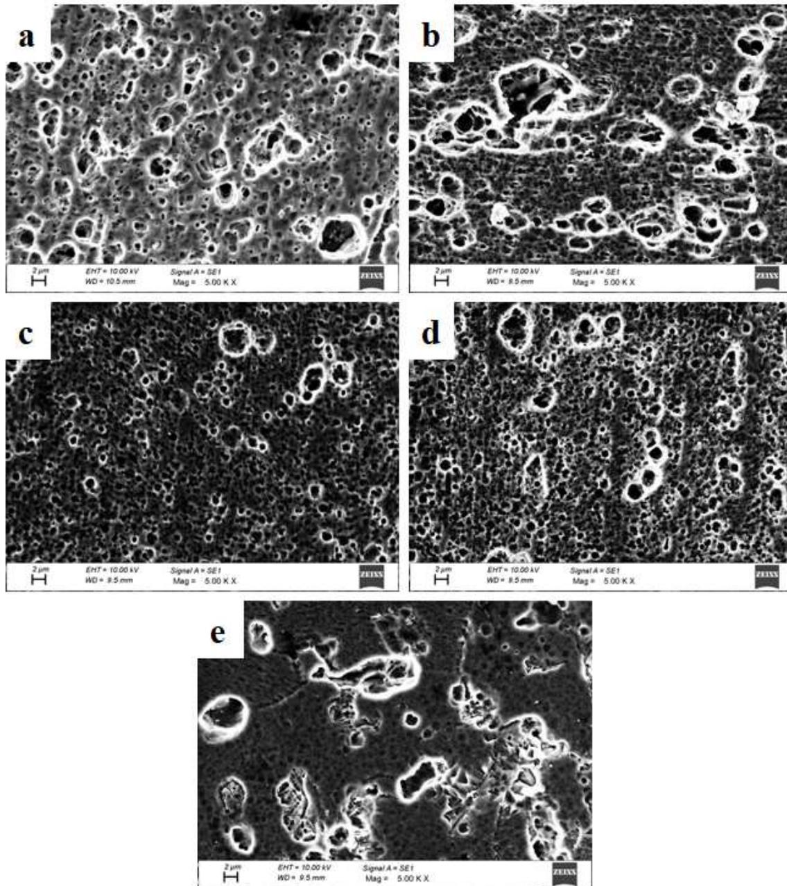
Fig. 2. Scanning Electron Microscopy (a) AA5083 Base Material (b) AA5754 Base Material (c) AA5083 HAZ (d) AA5754 HAZ (e) Weld Zone
