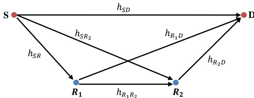
Figure 2: Three hop relay network
