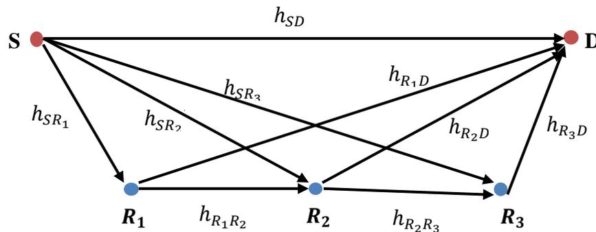
Figure 3: Four hop relay network
