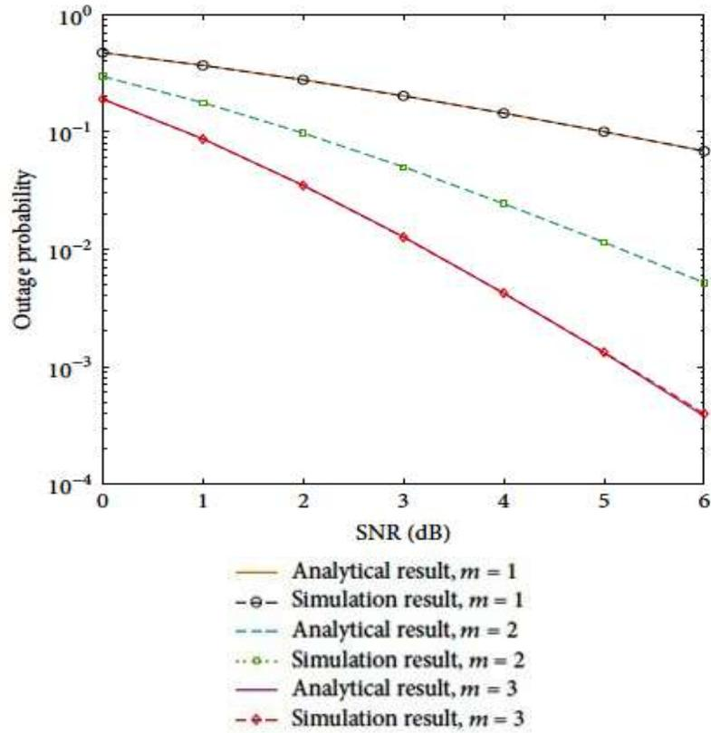
Figure 6: outage probability vs SNR by increasing relay nodes ( $m = 1, 2, 3$ )
