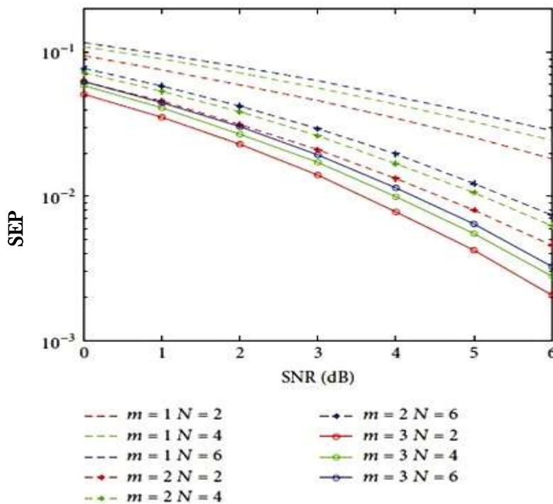
Figure 7: SEP vs SNR varying multiple links ( $m = 1, 2, 3$ ) and hops ( $N = 2, 4, 6$ ).
