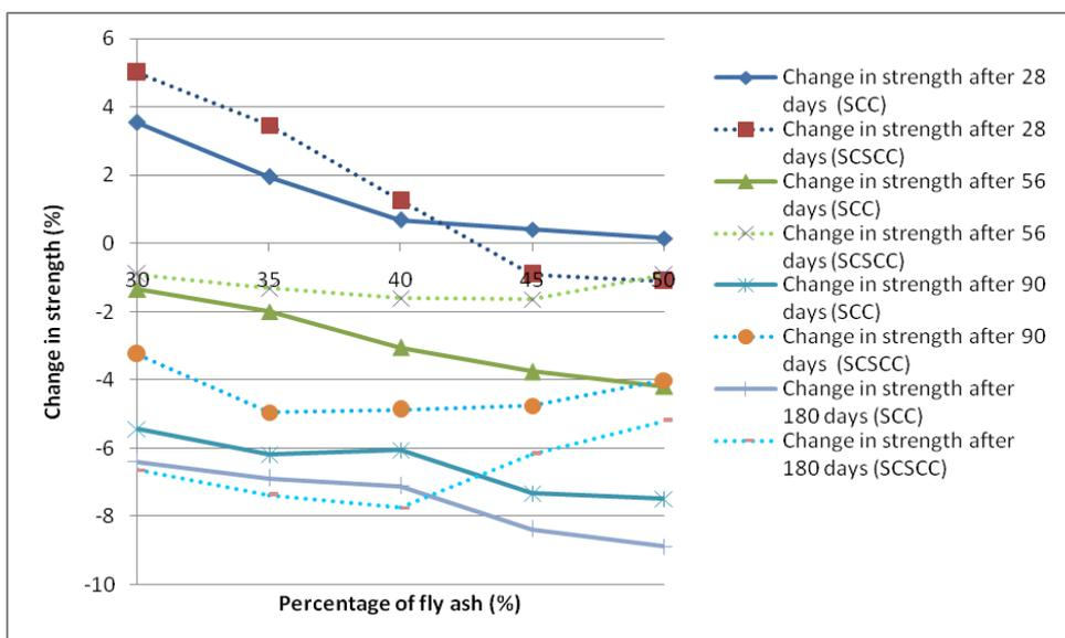
Figure 5(b) Change in strength after chloride exposure over time
