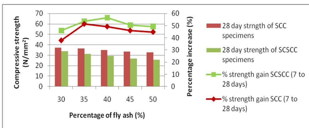
Figure 3 Compressive strength at 28 days & percentage increase from 7 to 28 days
