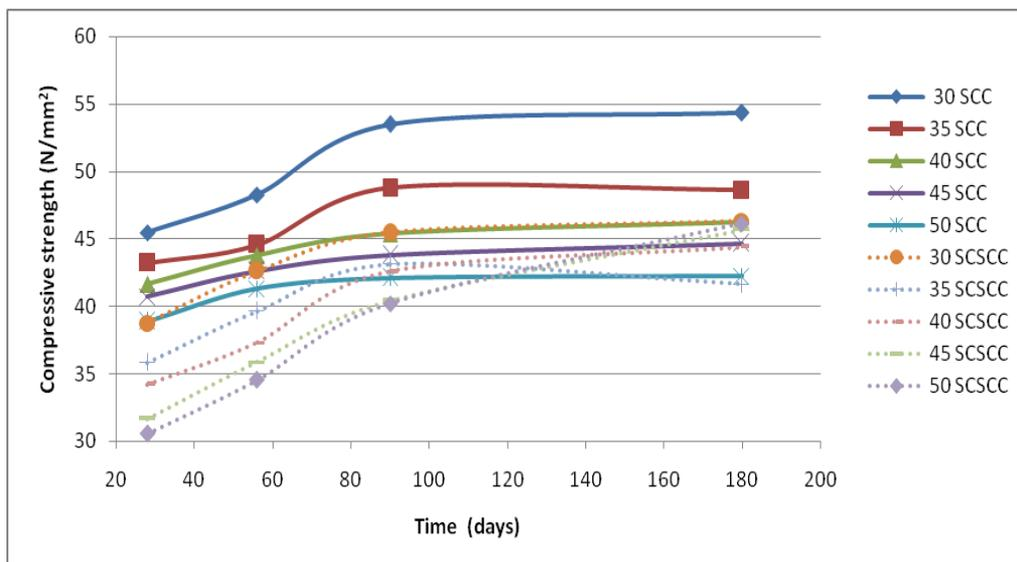
Figure 6(a). Compressive strength after immersion in sulphate solution
