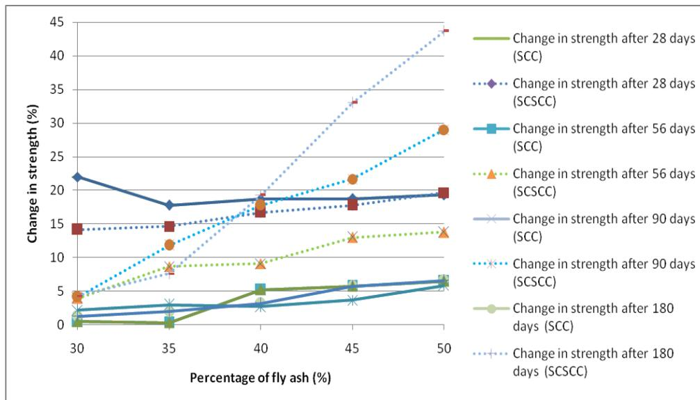
Figure 6(b) Change in strength on exposure to sulphate solution
