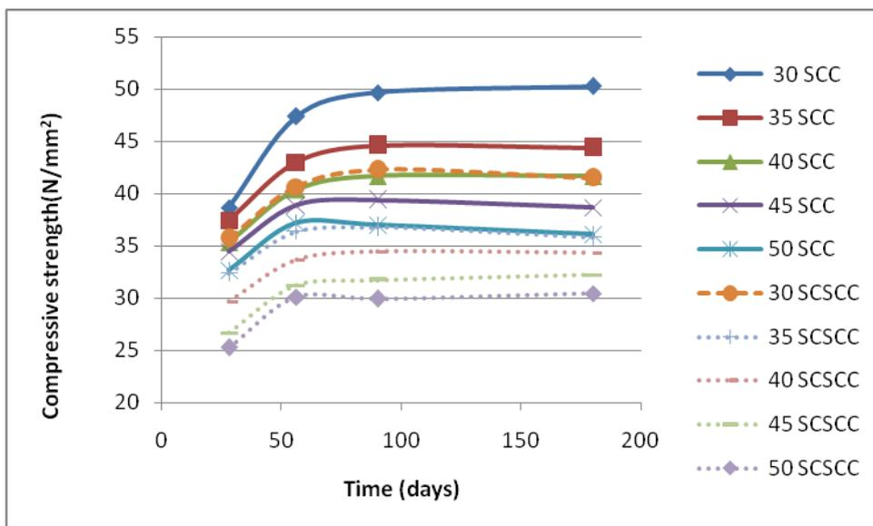
Figure 5 (a) Compressive strength after immersion in chloride solution
