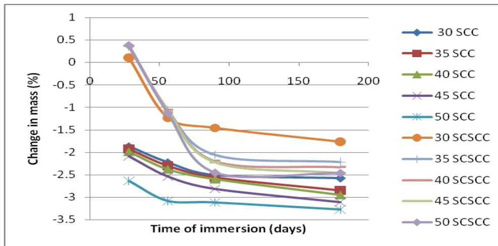
Figure 8 Change in mass after acid immersion
