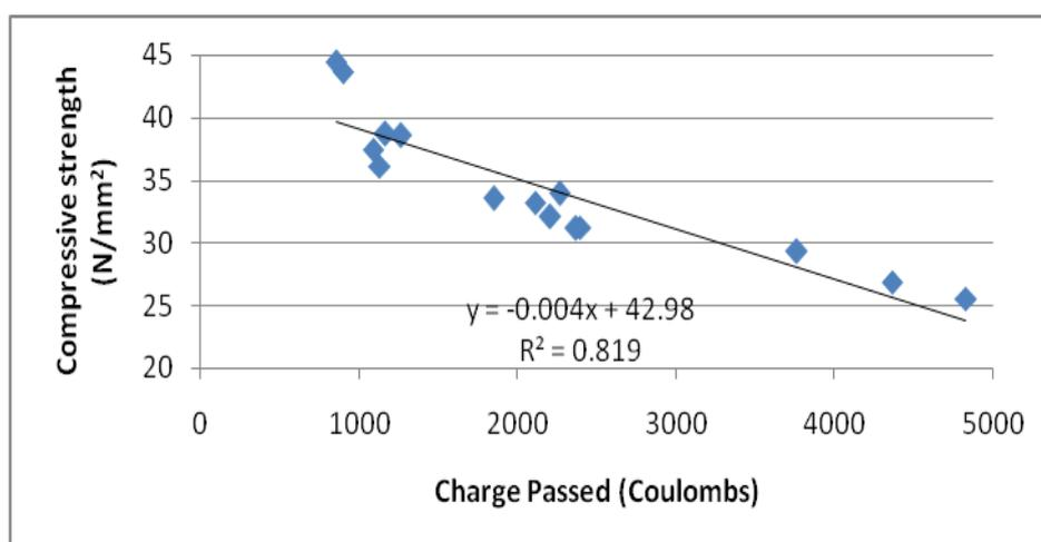
Figure 2 Relationship between compressive strength and charge passed
