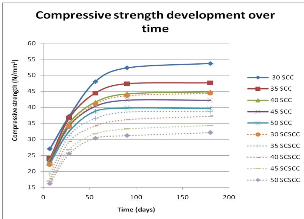
Figure 1 Compressive Strength Development over Time
