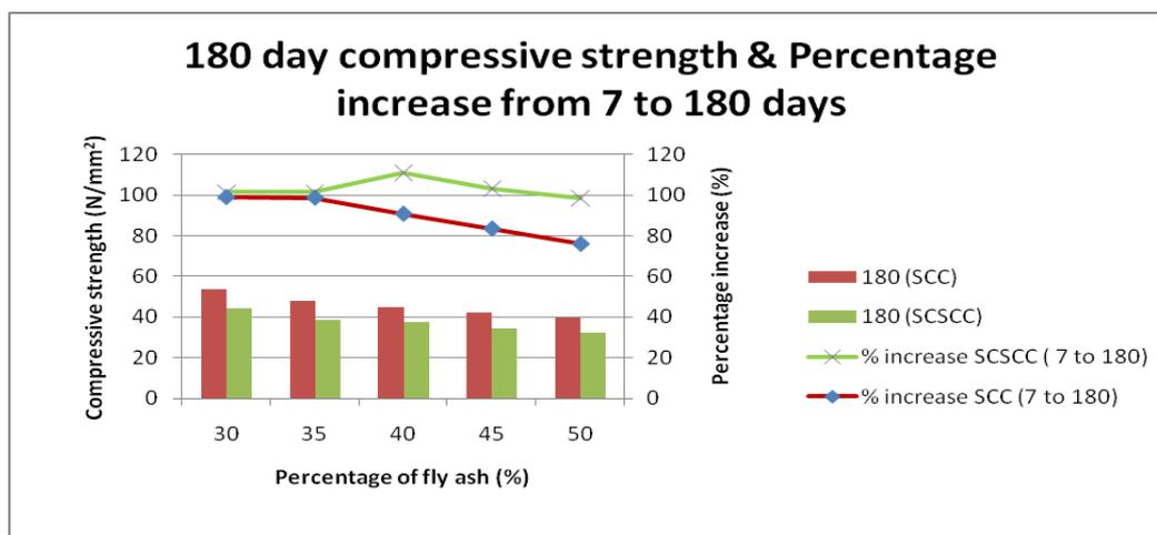
Figure 4. Compressive strength at 180 days & percentage increase from 7 to 180 days
