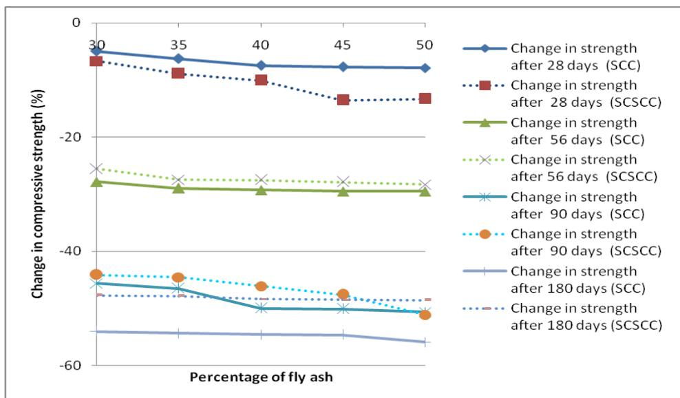
Figure 7 (b) Change in strength on exposure to acid solution over time
