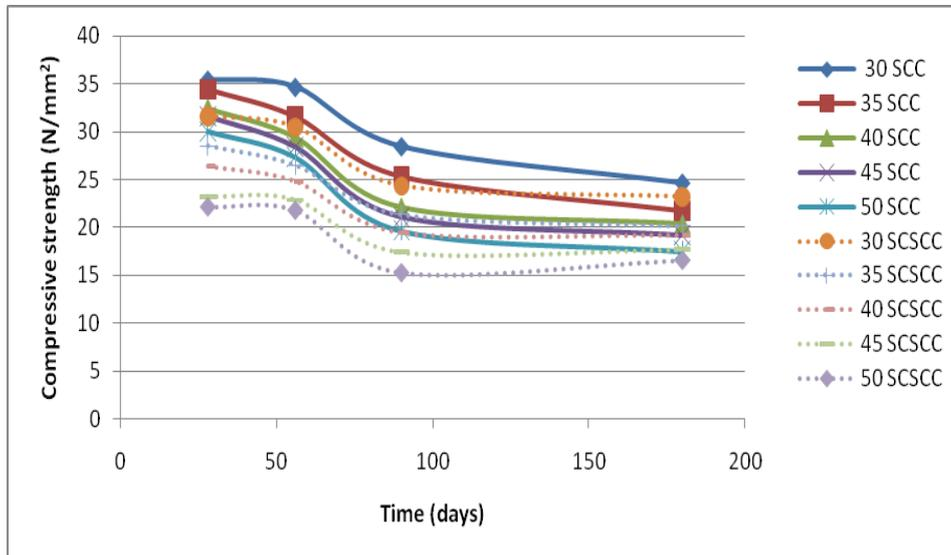
Figure 7(a) Compressive strength after immersion in acid solution
