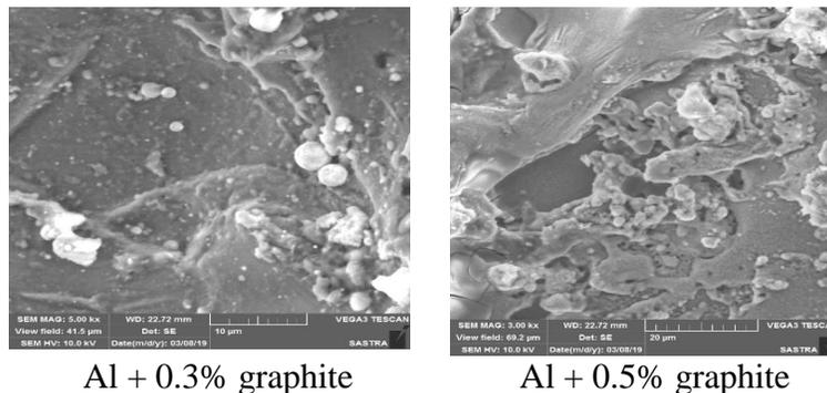
**Fig. 3 SEM Micrographs of aluminum graphite**
