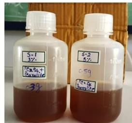
Fig. 2 Nanoparticles blended lubricant
