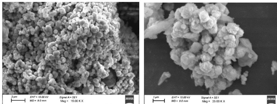
(a)  $\alpha$ -Fe<sub>2</sub>O<sub>3</sub>                      (b)  $\alpha$ -Fe<sub>2</sub>O<sub>3</sub> loaded Perlite
