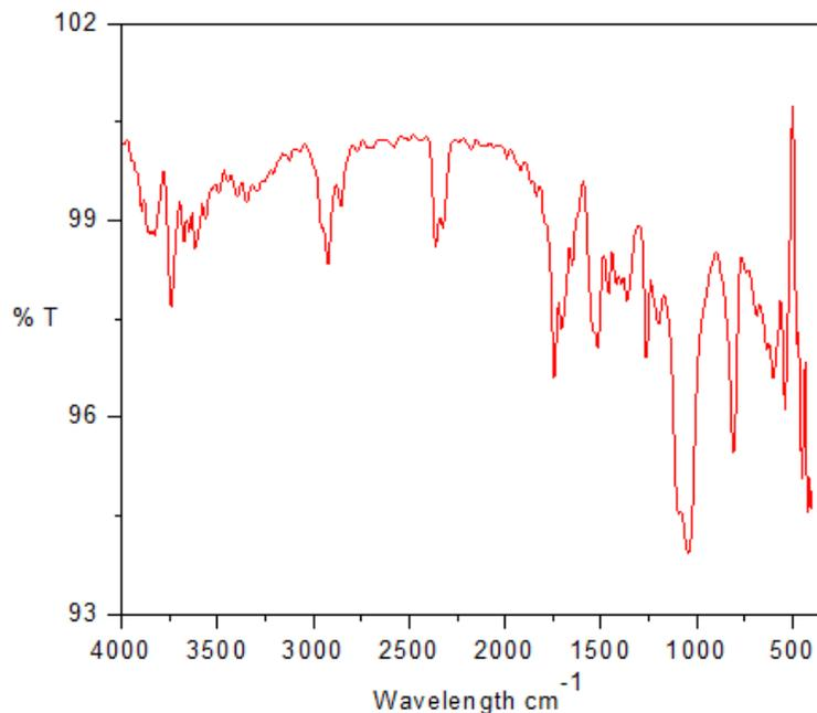
**Fig. 7 Fe<sub>2</sub>O<sub>3</sub> + perlite IR graph**
