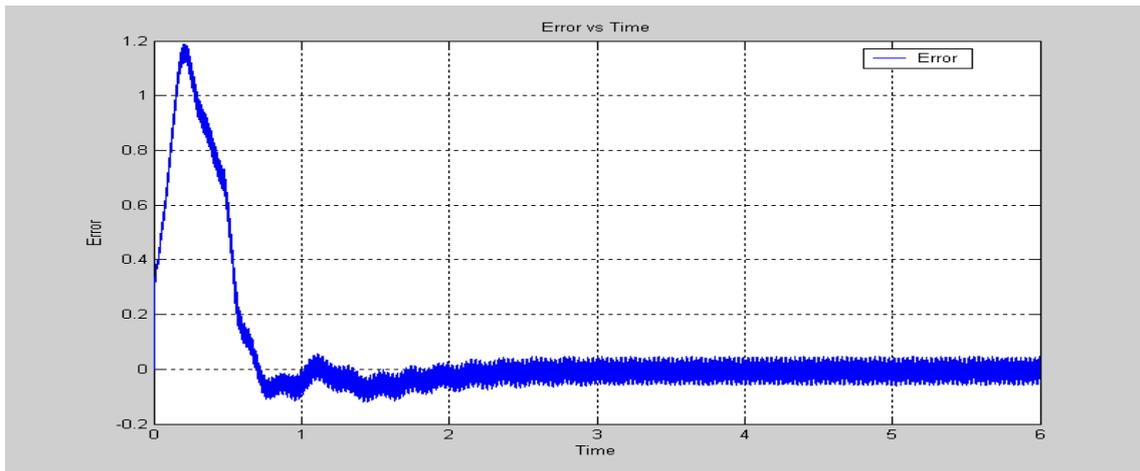
Figure 12: Flux Error between the Adjustable and Reference Model
