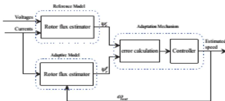
Figure 4b: Rotor Flux based MRAS
