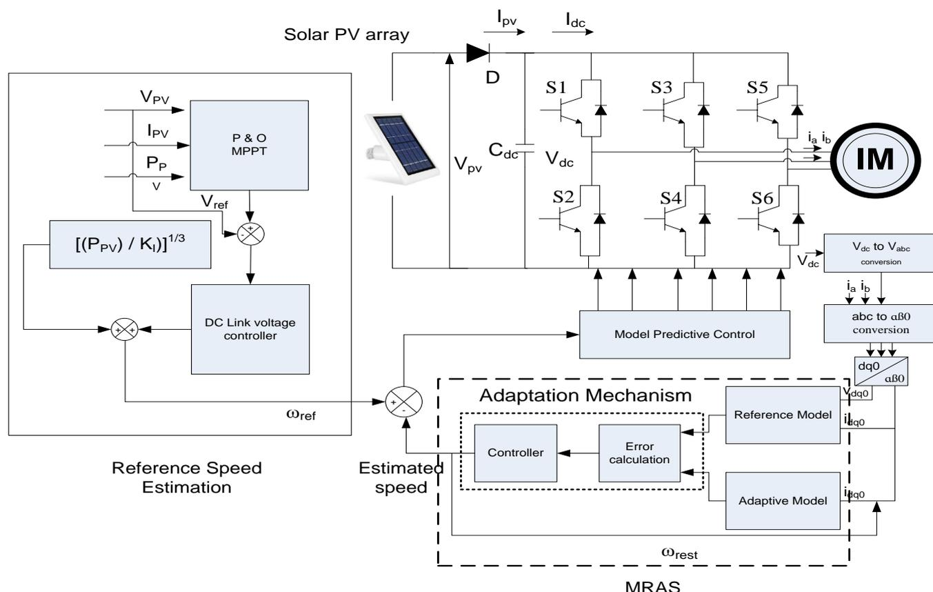
Figure 1: PV fed induction motor drive using Model predictive control
