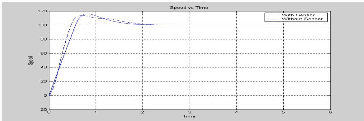
**Figure 10: Rotor speed by using MRAS 100 RPM**
