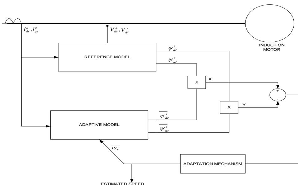
Figure 5: Block diagram of MRAS model for Induction Motor
