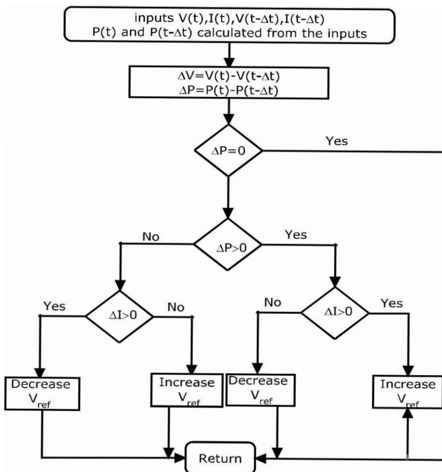
**Figure 3: Perturb and Observe Algorithm Flow Chart**
