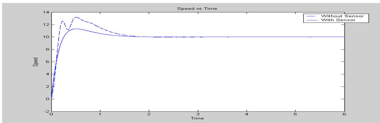
**Figure 11: Rotor speed by using MRAS at 10 RPM**
