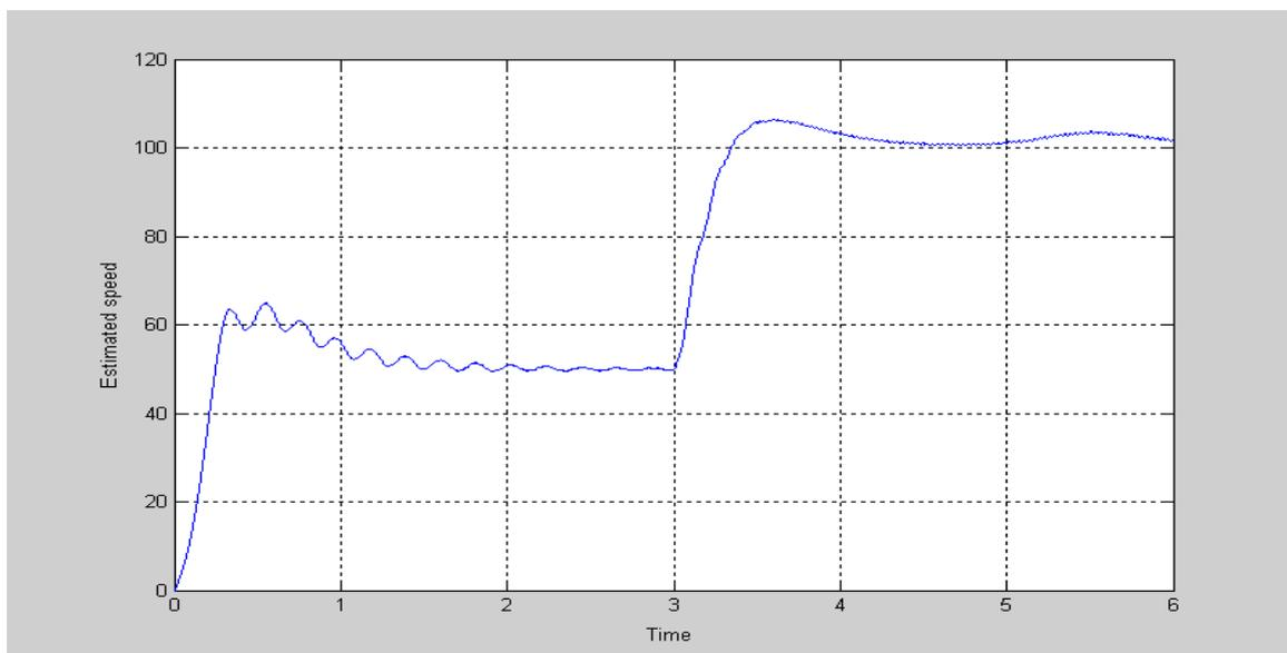
Figure 14: Step change in Reference speed from 50 rad/sec to 100 rad/sec
