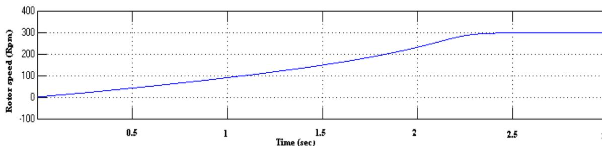
**Figure 7: Rotor speed by using MRAS at 305 RPM**
