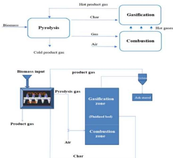
**Figure 3. Stages of Gasification**
