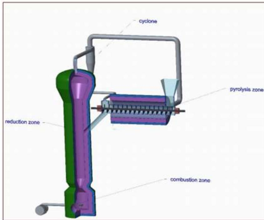
**Figure 4. System design indicating its three zones**
