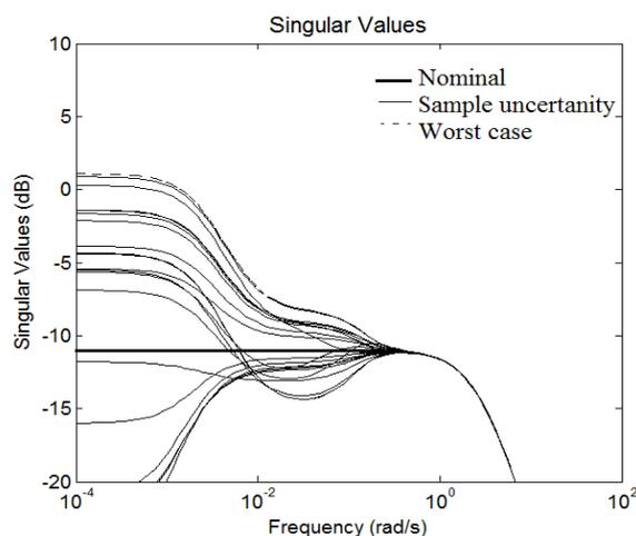
**Figure 10. Robustness Analysis Using Singular Values**
