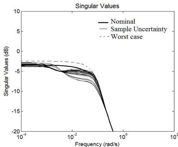
**Figure 13. Robustness Analysis Using Singular Values**
