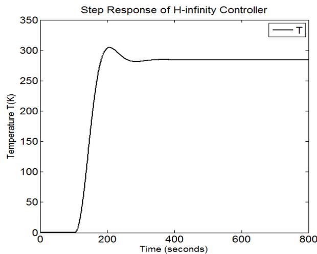
Figure 8. Temperature Response of H-Infinity Controller
