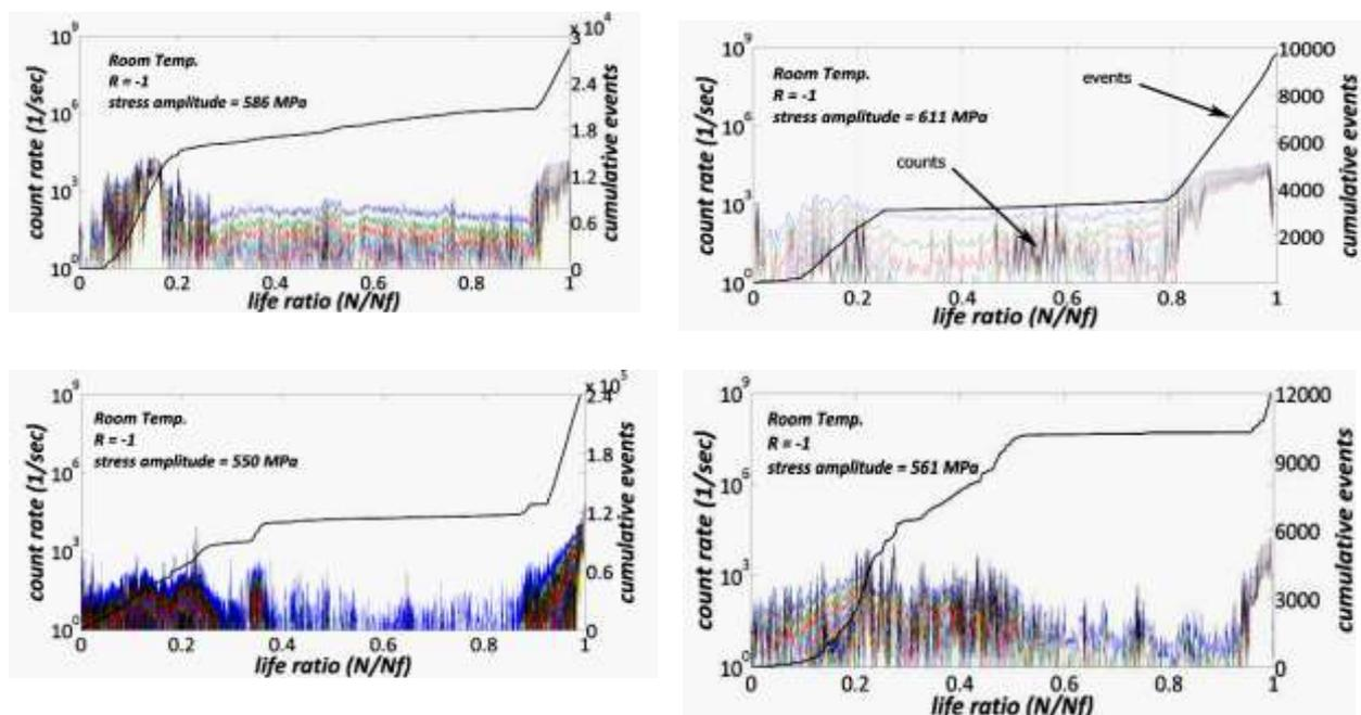
**Figure 5. Count Rate and cumulative events behavior at different stress amplitude levels**
