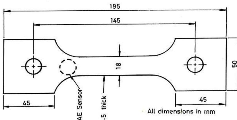
Figure 1. Tensile test Specimens
