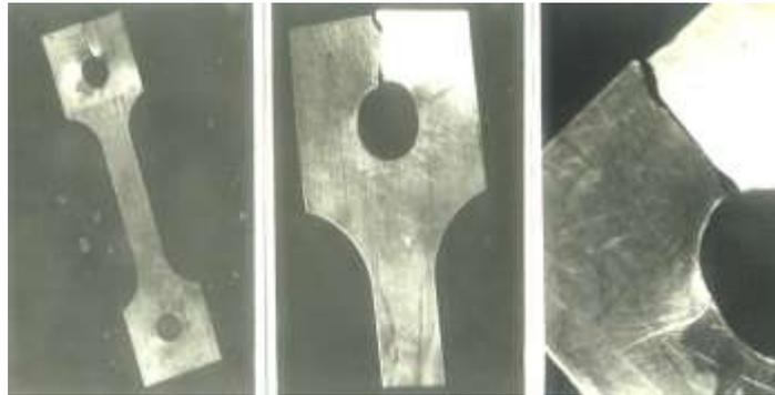
**Figure 2. Typical fractured tensile specimen**
