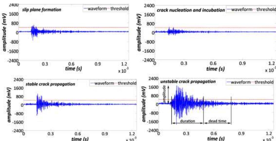
**Figure 8. Typical waveforms coming from the different stages**
