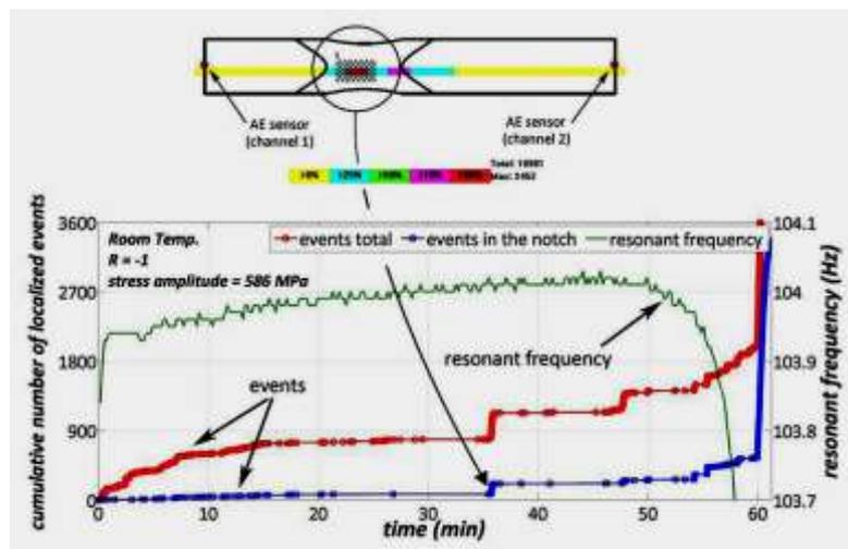
**Figure 6. Events and resonant frequency of RUMUL machine during fatigue test (Nf = 3. 84 x 10<sup>5</sup> cycles)**
