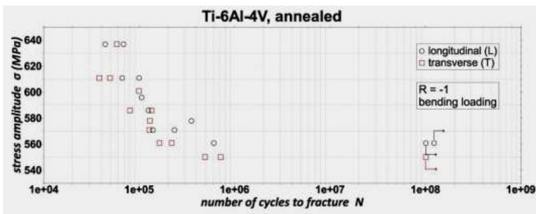
Figure 4. S-N diagram of specimens cyclically stressed in direction L and T of Ti-6Al-4V alloy
