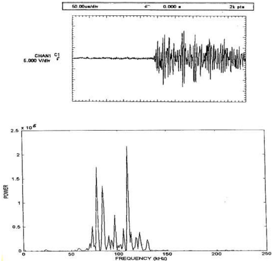
Figure 12. FFT Spectra for power vs. frequency at 15000 N Applied load
