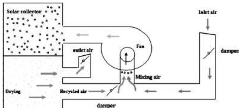
**Fig.7. Model Design of Hybrid Solar -Biomass system**
