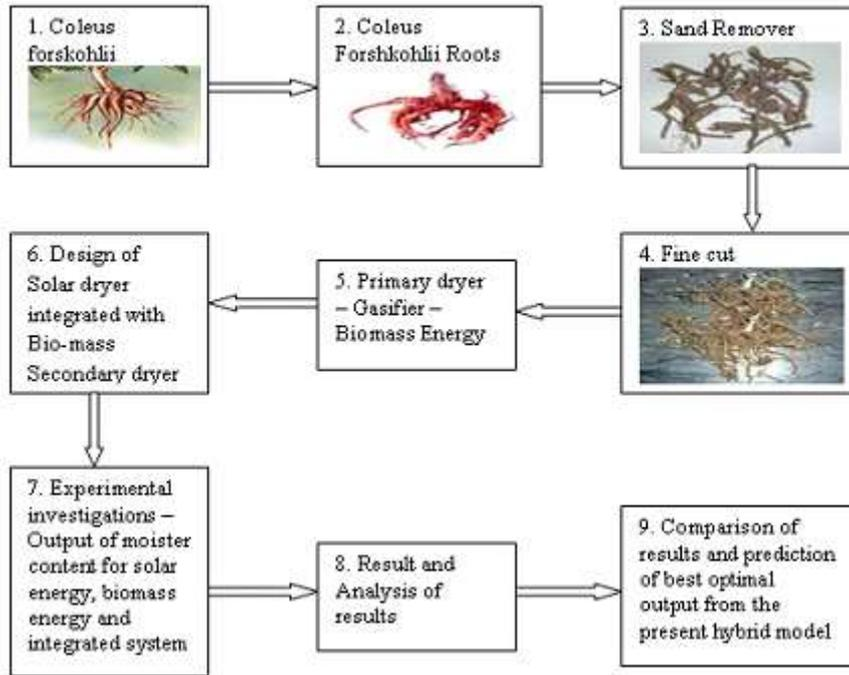
**Fig.4. Work sequence of proposed Hybrid system**
