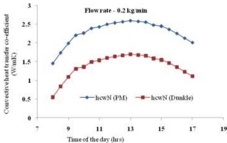
Fig.22 Variation of convective heat transfer coefficient of North facing wick surface
