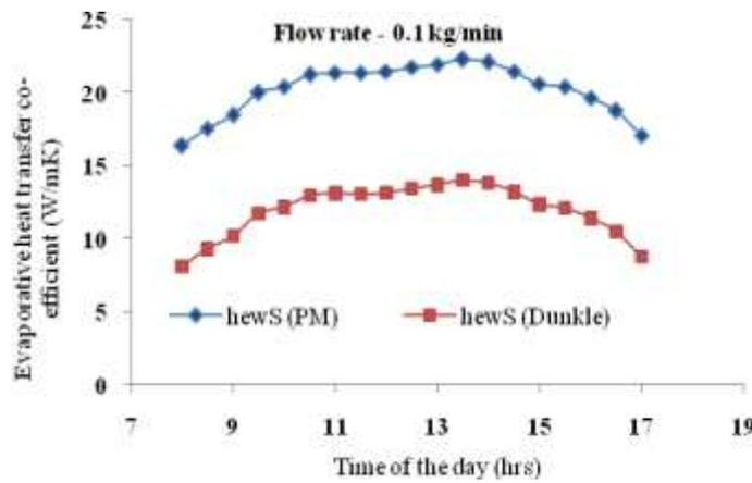
Fig. 15 Variation of evaporative heat transfer coefficient of South facing wick surface
