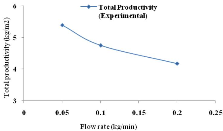
Fig. 35 Total productivity with respect to flow rate
