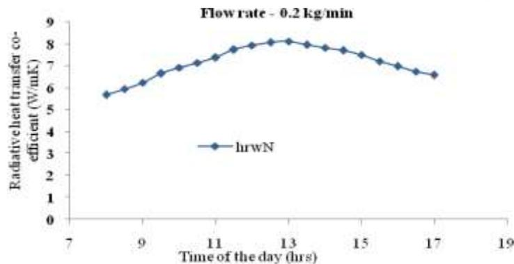
Fig.26 Variation of Radiative heat transfer coefficient of North facing wick surface
