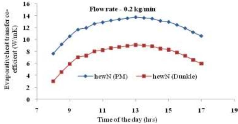
Fig.23 Variation of evaporative heat transfer coefficient of South facing wick surface
