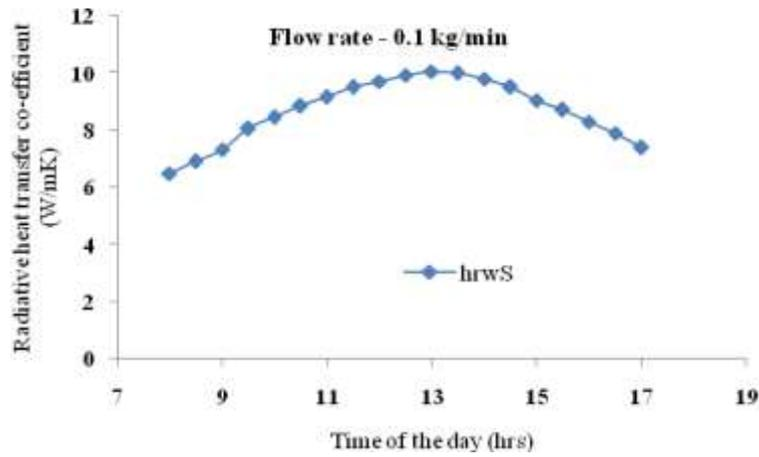
Fig.17 Variation of Radiative heat transfer coefficient of South facing wick surface
