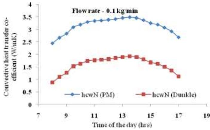
Fig. 14 Variation of convective heat transfer coefficient of North facing wick surface
