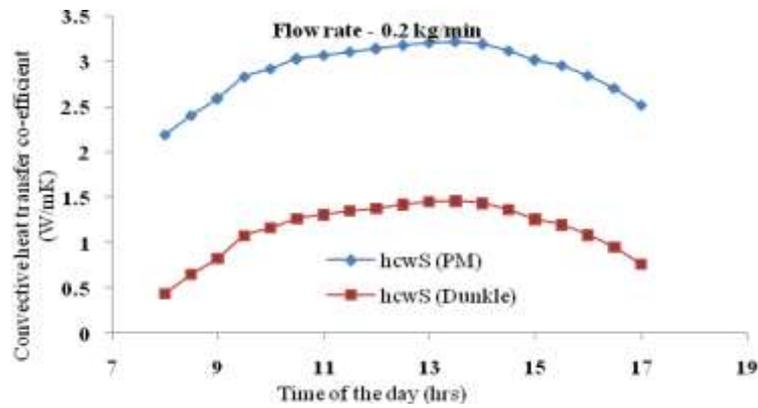
Fig.21.Variation of convective heat transfer coefficient of South facing wick surface
