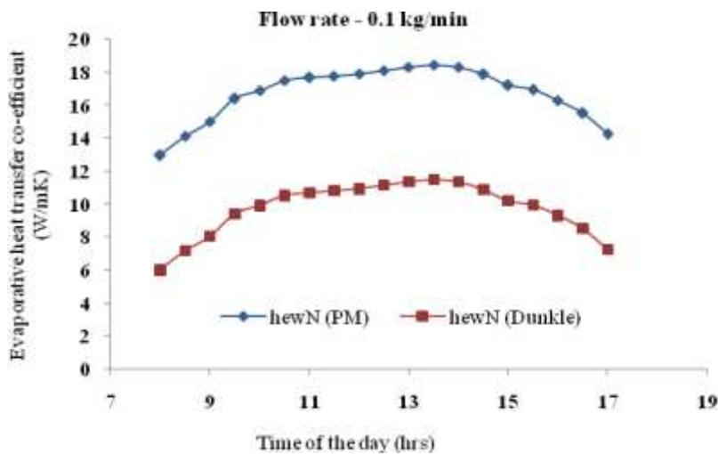
Fig.16 Variation of evaporative heat transfer coefficient of North facing wick surface
