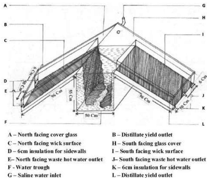
Fig. 1 Schematic sectional view of the proposed still
