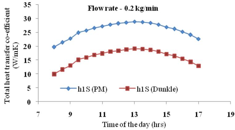
Fig .27 Variation of total heat transfer coefficient of South facing wick surface
