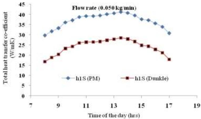
Fig. 11 Variation of total heat transfer coefficient of South facing wick surface
