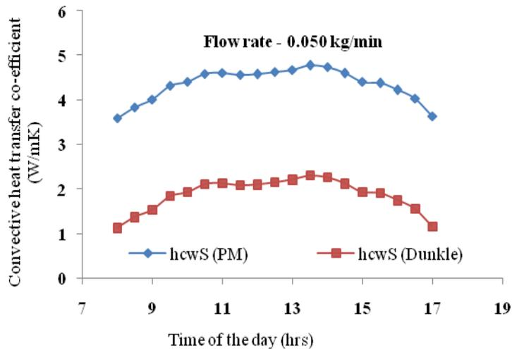
Fig .5 Variation of convective heat transfer coefficient of South facing wick surface
