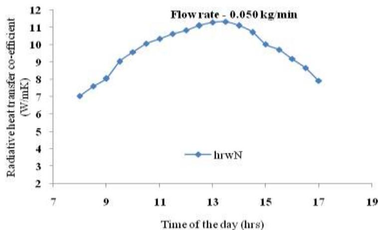
Fig.10 Variation of radiative heat transfer coefficient of North facing wick surface
