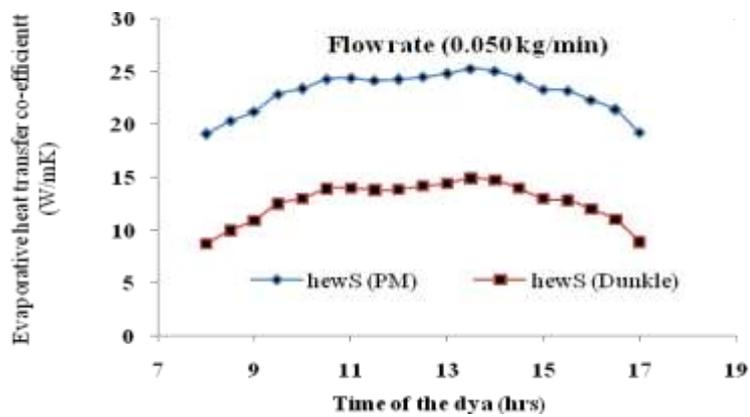
Fig .7 Variation of evaporative heat transfer coefficient of south facing wick surface
