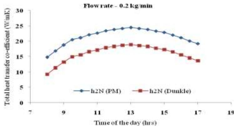
Fig .28 Variation of total heat transfer coefficient of North facing wick surface
