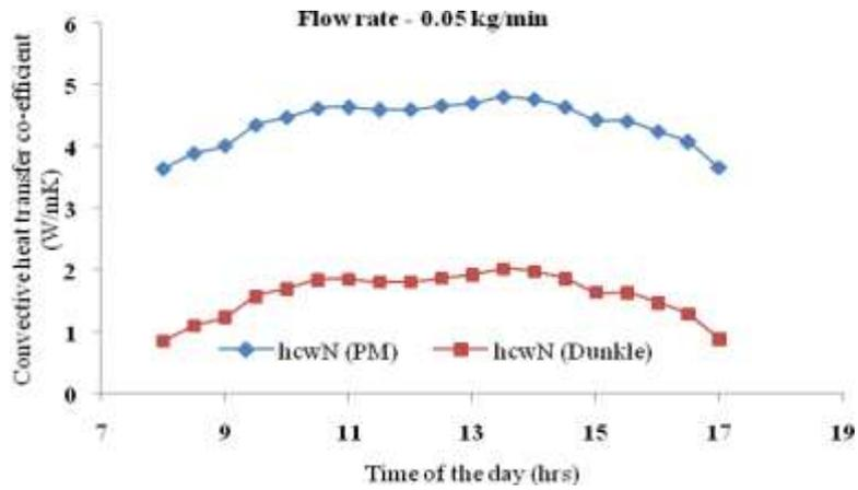
Fig .6 Variation of convective heat transfer coefficient of North facing wick surface
