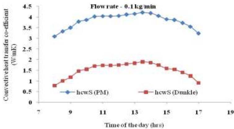
Fig.13 Variation of convective heat transfer coefficient of South facing wick surface
