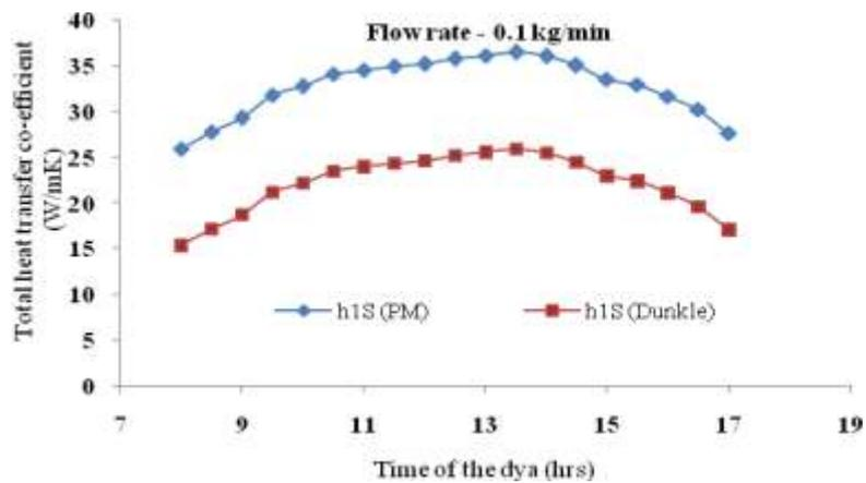
Fig.19 Variation of total heat transfer coefficient of South facing wick surface
