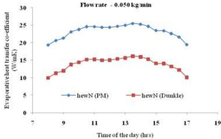
Fig.8 Variation of evaporative heat transfer coefficient of North facing wick surface
