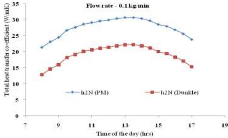
Fig.20 Variation of total heat transfer Coefficient of North facing wick surface
