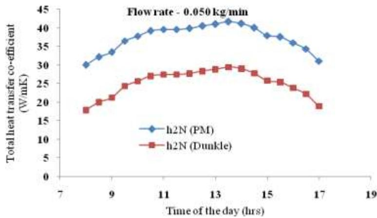
Fig.12 Variation of total transfer coefficient of North facing wick surface
