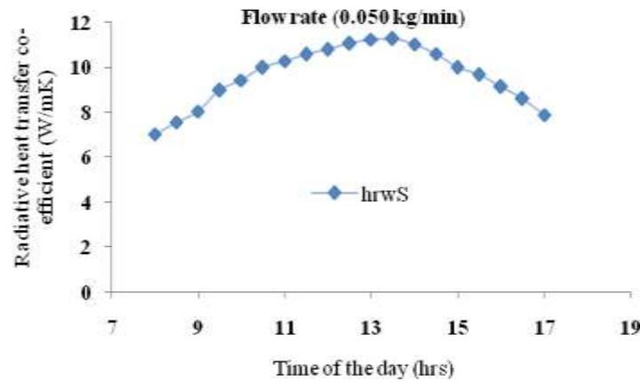
Fig. 9 Variation of Radiative heat transfer coefficient of South facing wick surface
