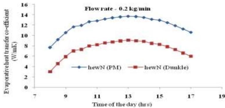
Fig.24 Variation of evaporative heat transfer coefficient of North facing wick surface
