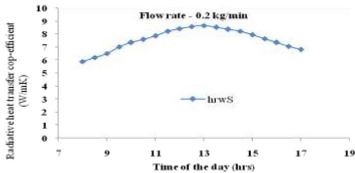
Fig.25 Variation of Radiative heat transfer coefficient of South facing wick surface
