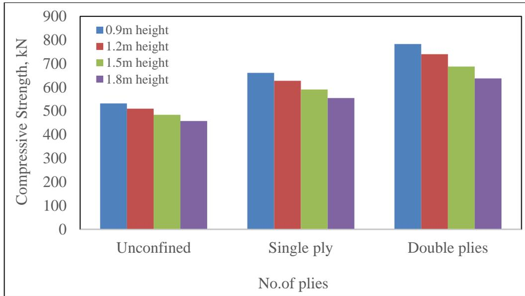
**Fig. 2.** Effect of height of square CFT column on compressive load capacity
