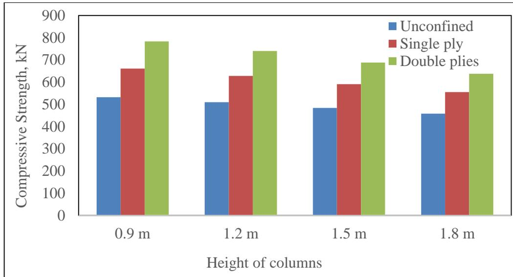
**Fig. 3.** Strength in compression of square CFT columns confined with single as well as double plies of GFRP
