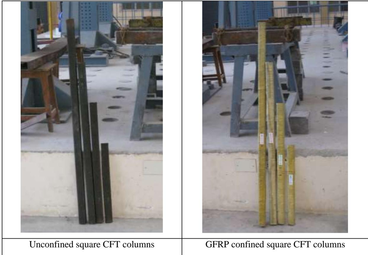
**Fig. 1.** GFRP confined and unconfined square CFT columns
