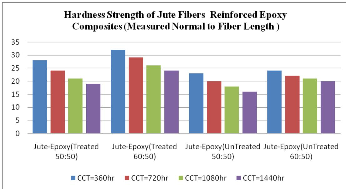
Figure 3 shows the hardness strength of composites (Measured normal to fiber length)
