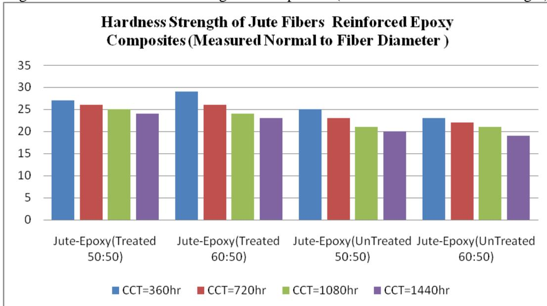
Figure 4 shows the hardness strength of composites (Measured normal to fiber diameter)
