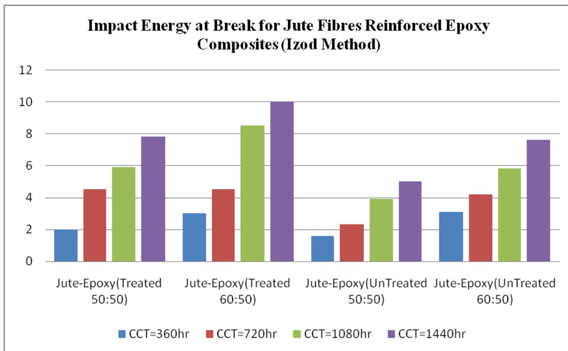
Figure 2 Shows impact energy of composites in Izod impact test
