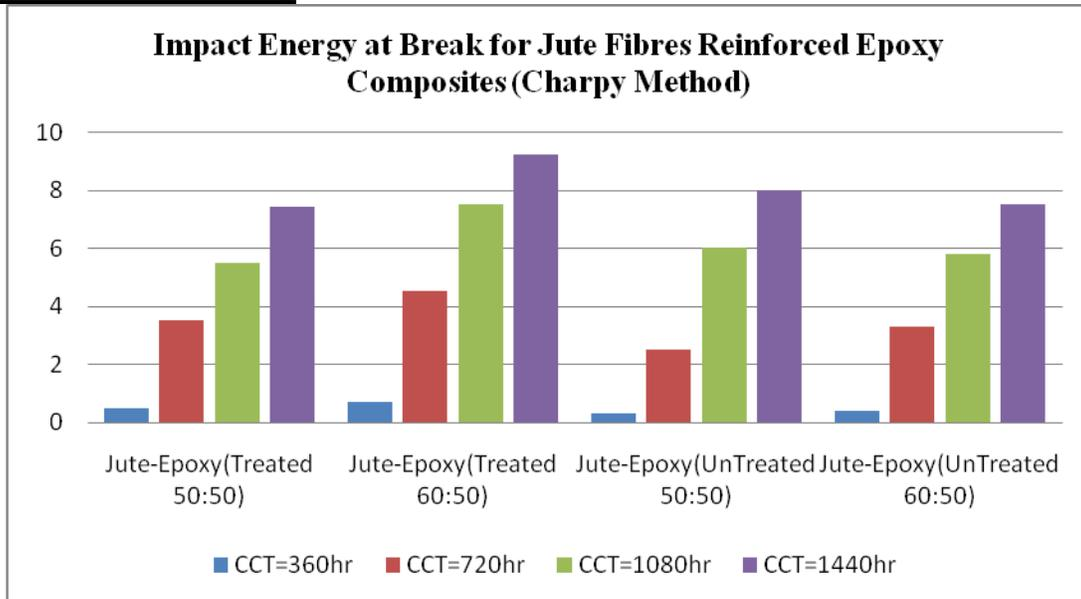
Figure 1 Shows impact energy of composites in charpy impact test
