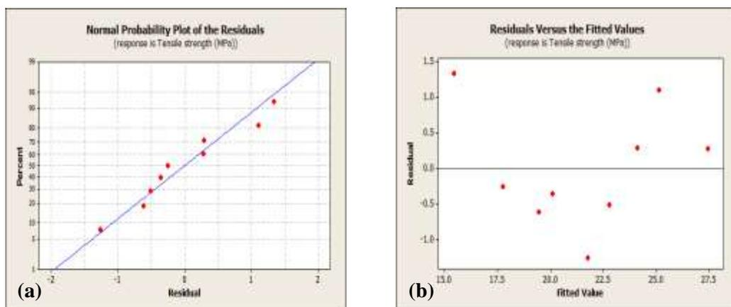
Figure 1 Residual analysis in tensile strength (a) normal probability plot of the residuals, and (b) the residuals versus the fitted (predicted response) values
