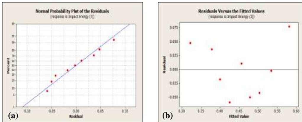
Figure 4 Residual analysis in impact energy (a) normal probability plot of the residuals, and (b) the residuals versus the fitted (predicted response) values
