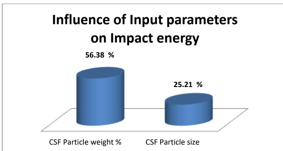
Figure 12 Influence of Input parameters on impact energy
