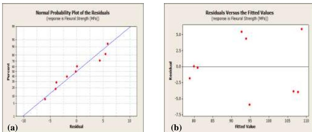
Figure 2 Residual analysis in flexural strength (a) normal probability plot of the residuals, and (b) the residuals versus the fitted (predicted response) values
