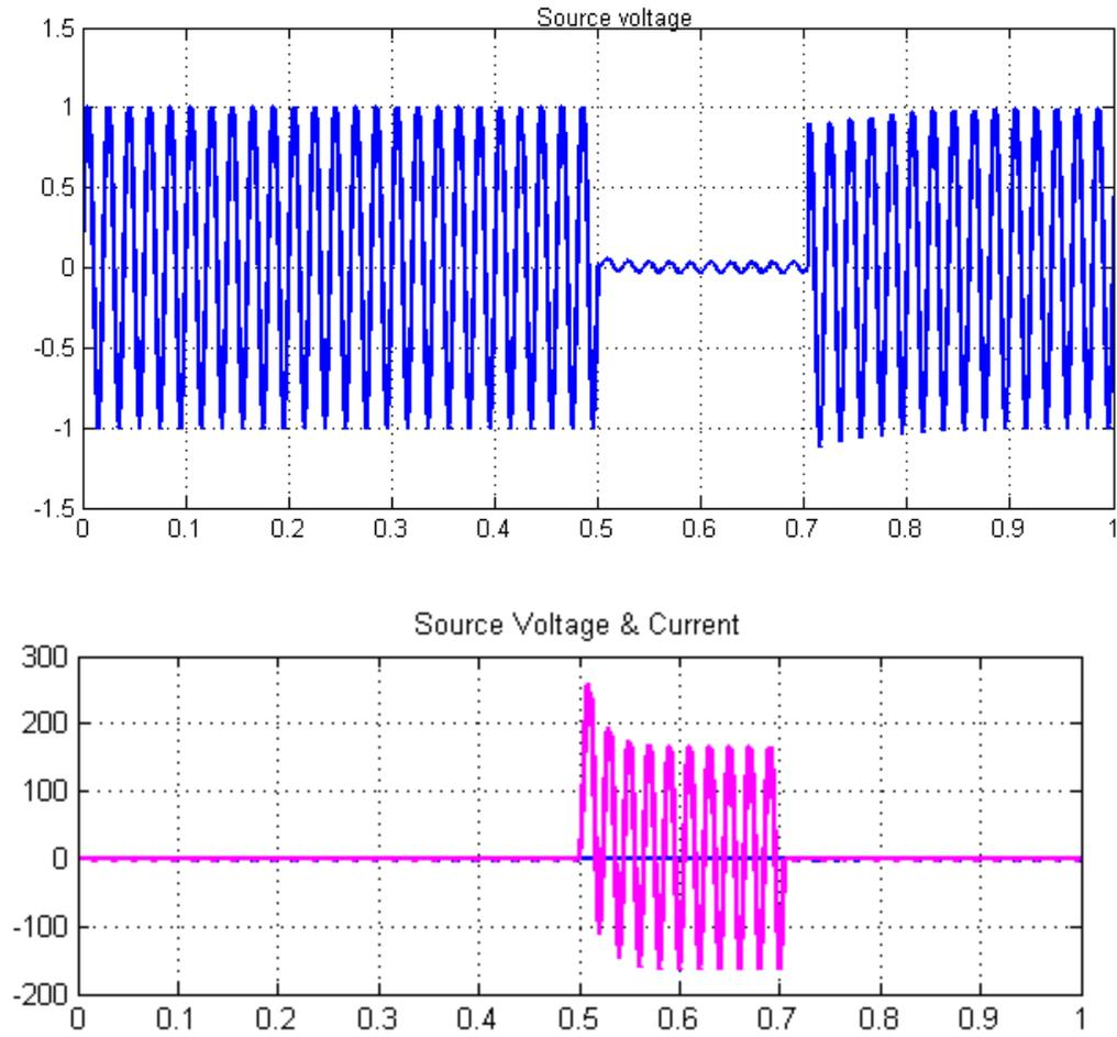
Fig. 3 Source voltage and Source current with sag
