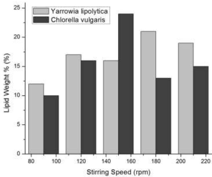
Figure 4: Effect of Stirring Speed on Lipid Weight
