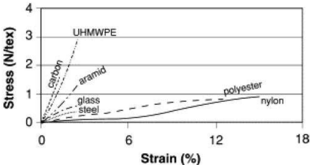
Figure 2: Stress/strain charts of various fibers.
