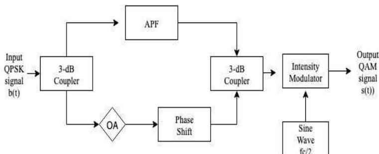
**Figure. 4. Schematic diagram of modulation format conversion from QPSK to 16-QAM**
