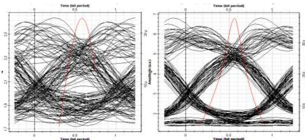
**Figure. 9. Eye diagram without dispersion compensation and after dispersion compensation.**
