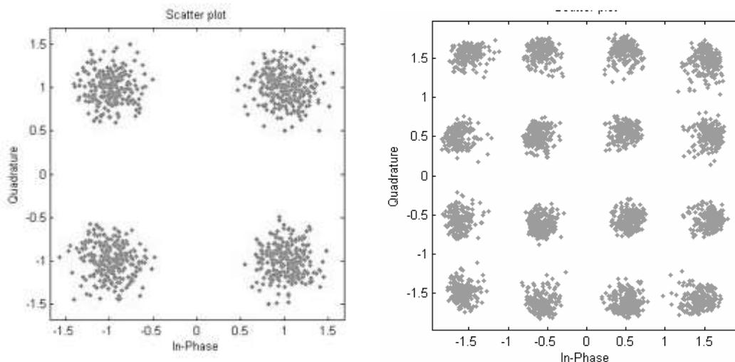
**Figure.8. Constellation diagram of QPSK and 16-QAM signals after modulation format conversion using APF**
