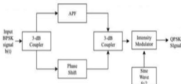
Figure. 3. Structure of BPSK to QPSK converter using APF whose delay is  $\Delta T$ .
