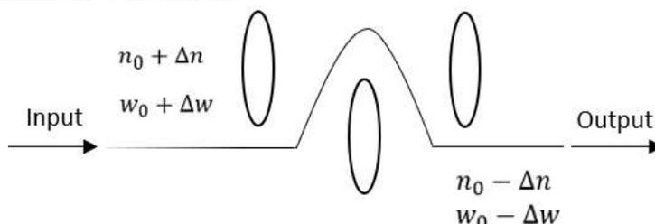
**Figure. 1. Balanced SCISSOR three stage All Pass Filter.**
