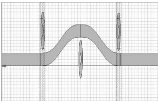
Figure. 2. Waveguide design of three stage APF using OptiBPM.
