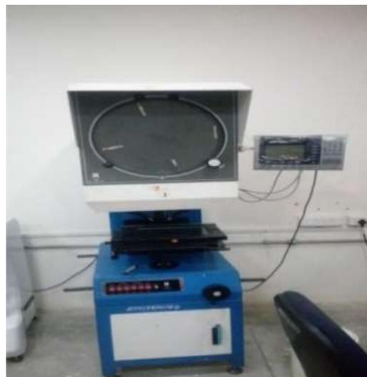
**Figure 4. Digital optical profile projector**
