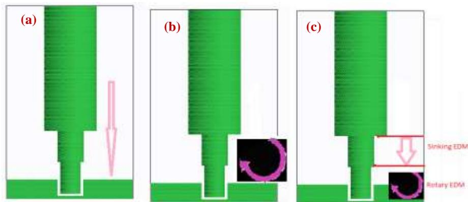
**Figure 2. Electrode configuration (a) Sinking electrode method (Step -1 & 2), (b) Rotary electrode method (Step -1 & 2) and (c) Combination Method ( Step-1- Rotary and Step-2- Sinking)**
