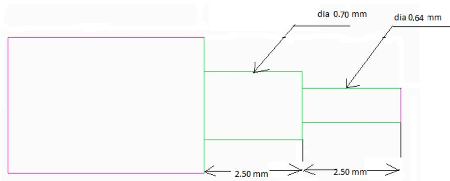
**Figure 1. Multi diameter electrode**
