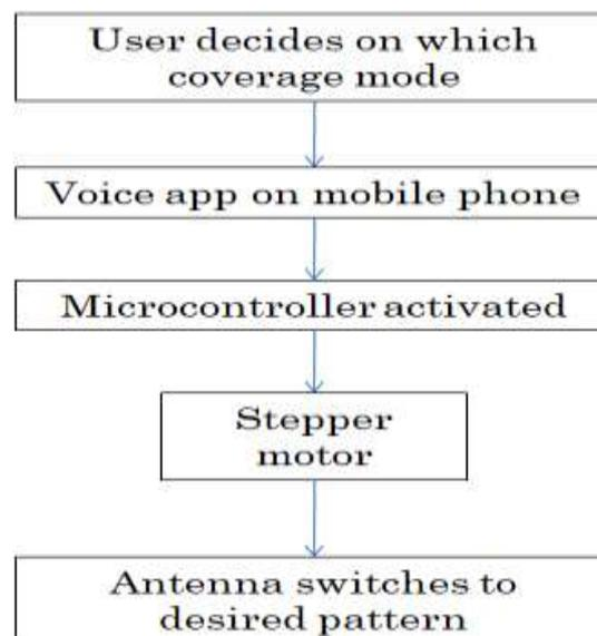
**Figure 3. Flow Diagram of The Proposed Antenna System**
