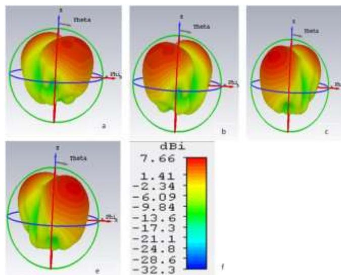
Figure 6. Dimensional Radiation Pattern of the MIMO Antenna
