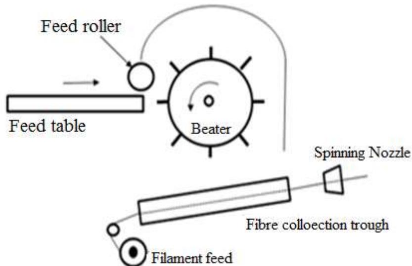
**Figure 1. Principle of mechanised coir spinning**
