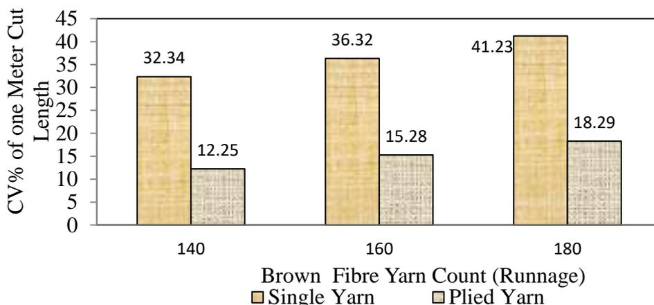
**Figure 11. CV% of one meter cut length of single and plied yarns made from brown fibre**
