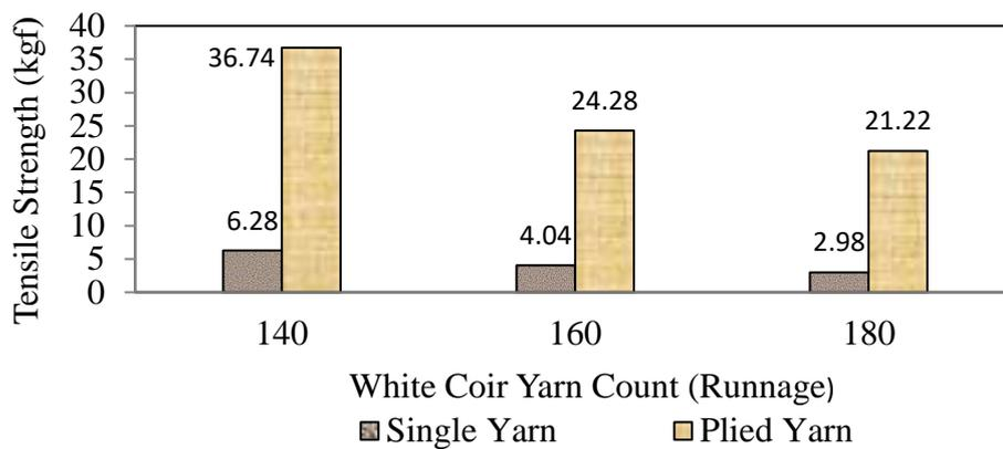
**Figure 6. Tensile strength of white fibre yarns**
