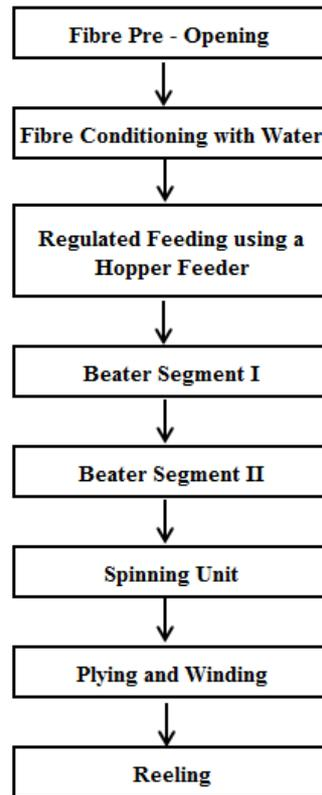
**Figure 2. Process flow of mechanised spinning**
