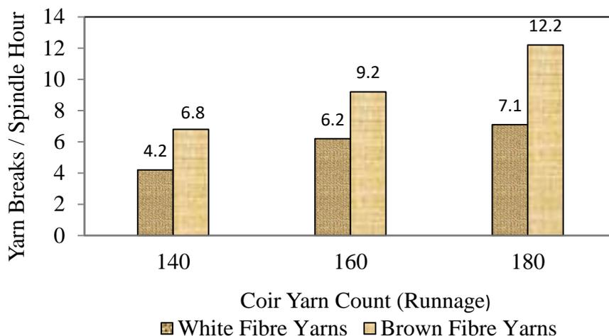
**Figure 12. Yarn breaks per spindle hour for white and brown fibre yarns**
