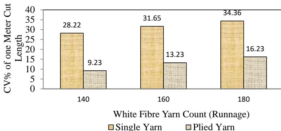
**Figure 10. CV% of one meter cut length of single and plied yarns made from white fibre**
