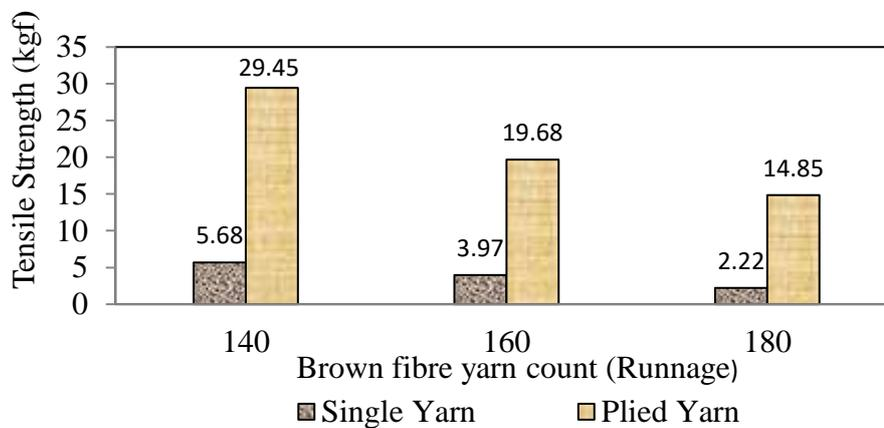
**Figure 7. Tensile strength of brown fibre yarns**
