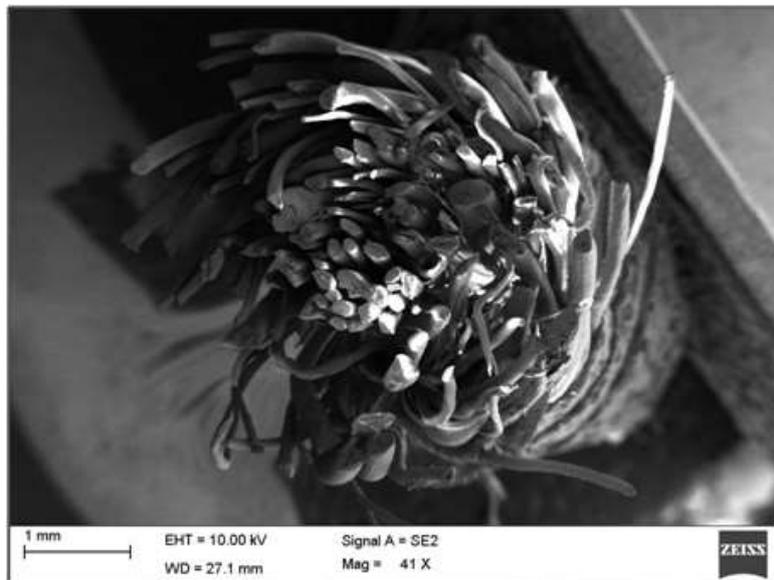
**Figure 3. Longitudinal image of mechanised spun single yarn**
