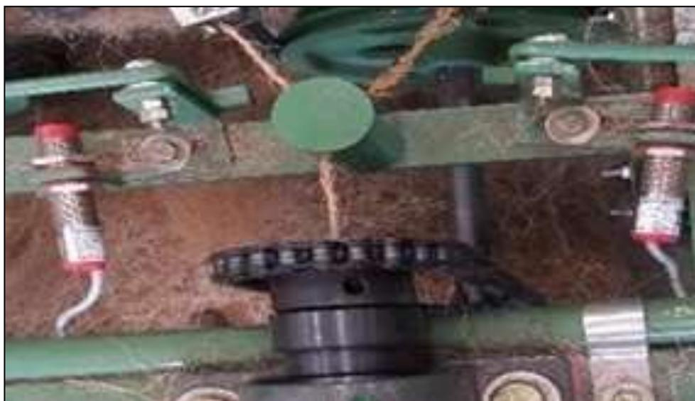
**Figure 5. Plying of single coir fibre yarns**
