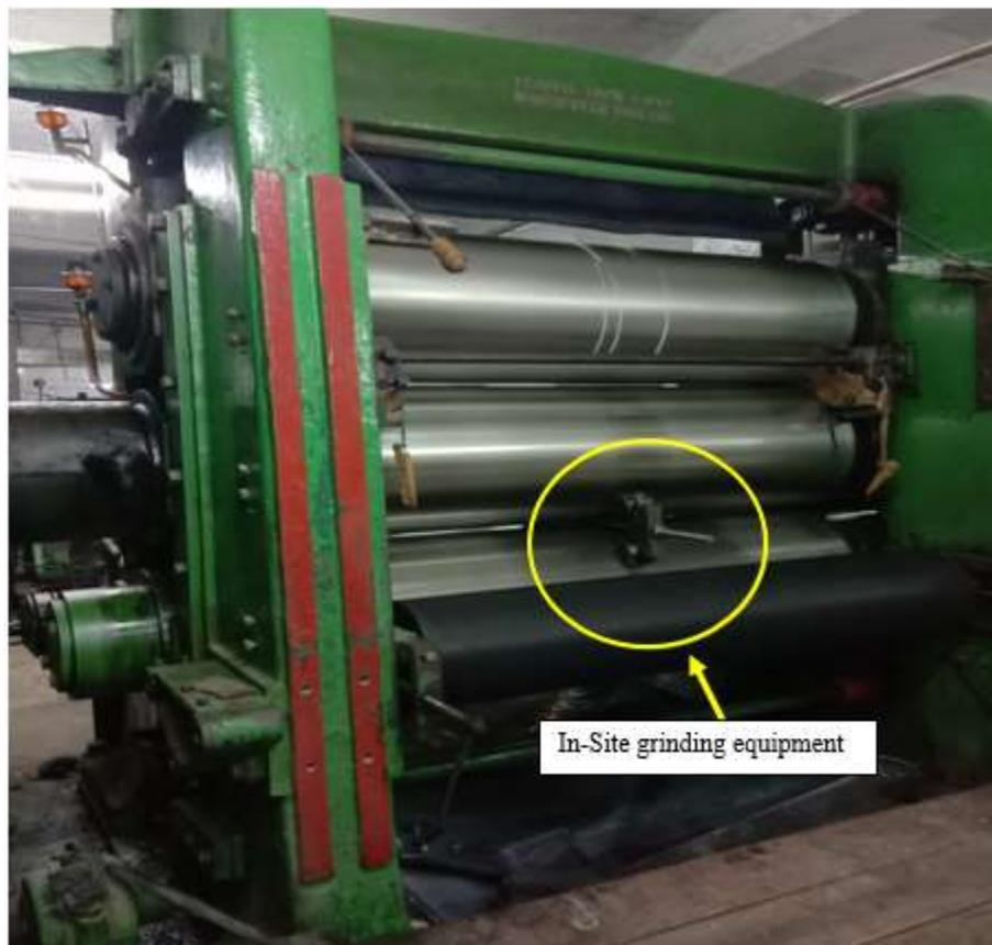
**Figure 1. Three roll calendar machine with in-site grinding equipment**
