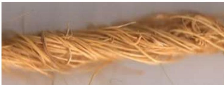
**Figure 3. Mechanised Spun Single Yarn**
