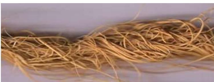
**Figure 4. Untwisted Mechanised Spun Single Yarn**
