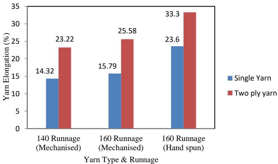
Figure 8. Elongation of Single and Two ply Coir Yarns
