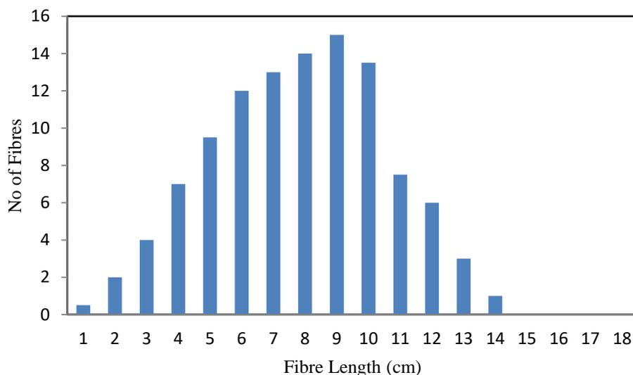
**Figure 6. Fibre Length Distribution in Mechanised Spun Single Yarn**
