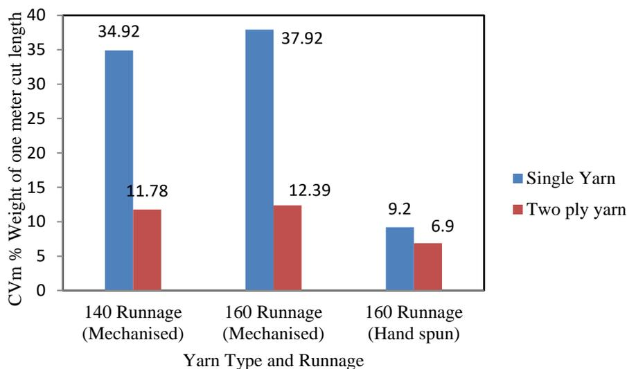
**Figure 9. CV% of One Meter Cut Length of Single and Two ply Coir Yarns**
