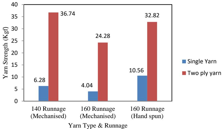
Figure 7. Tensile Strength of Single and Two ply Coir Yarns
