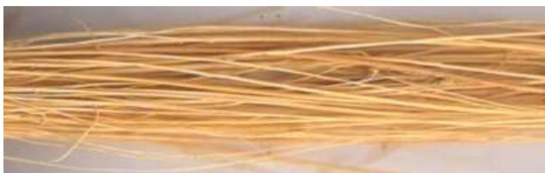
**Figure 2. Untwisted Hand Spun Single Yarn**
