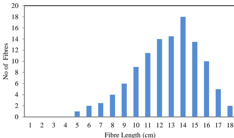
**Figure 5. Fibre Length Distribution in Hand Spun Single Yarn**
