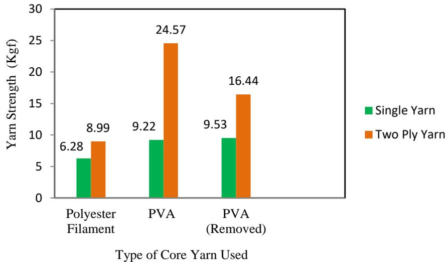
**Figure 10. Effect of Core Component on the Tensile Strength of Coir Yarns**
