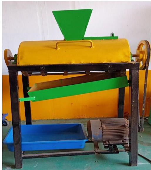
Figure 2. Power operated mango stone decorticator
